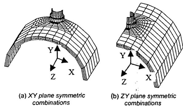
Figure 3: Finite element models for loading combinations
