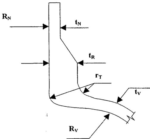
Figure 1: The studied nozzle to pressure vessel connection
