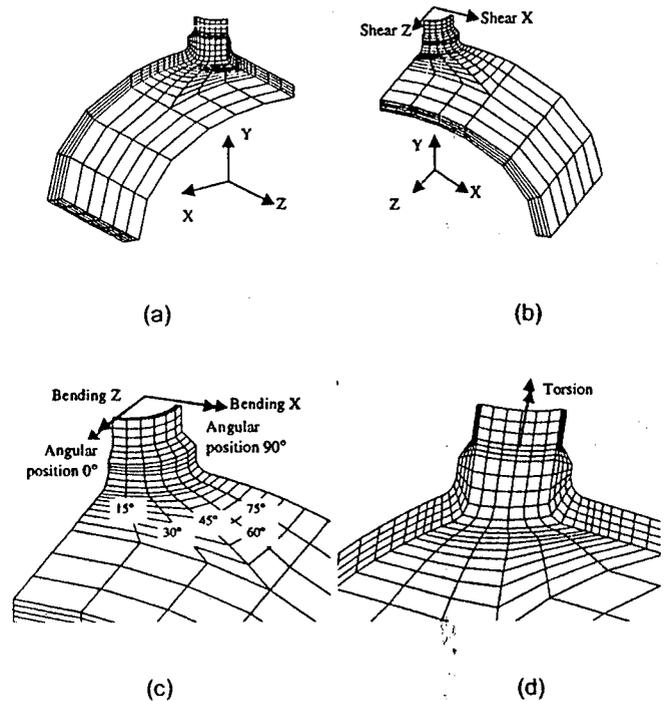
Figure 2: Details of the basic finite element model
