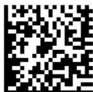
Figure 1. Example of the Data Matrix code [17].
