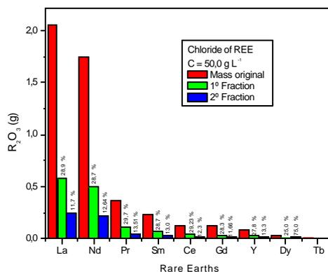
**Figure 4 – Fractionation of rare earths by dialysis at pH4, without stirring, using Nafion – 324 membranes.**
