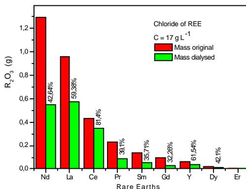
**Figure 2 – Fractionation of rare earths in pH 1, with stirring, using Ionac MC-3470XL membrane**
