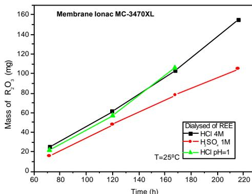
**Figure 1 – Behavior of some fractions of rare earths on Ionac membrane dialysis in hydrochloric and sulfuric media**
