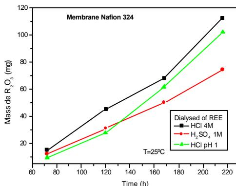
**Figure 3 - Behavior of dialysis of rare earths with Nafion membrane in hydrochloric and sulfuric media.**
