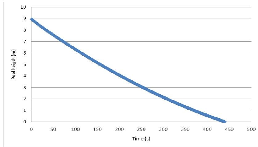
**Figura 7. Time to drain the reactor pool down to the level of the bottom of the core during a Primary Coolant Boundary Rupture postulated accident.**
