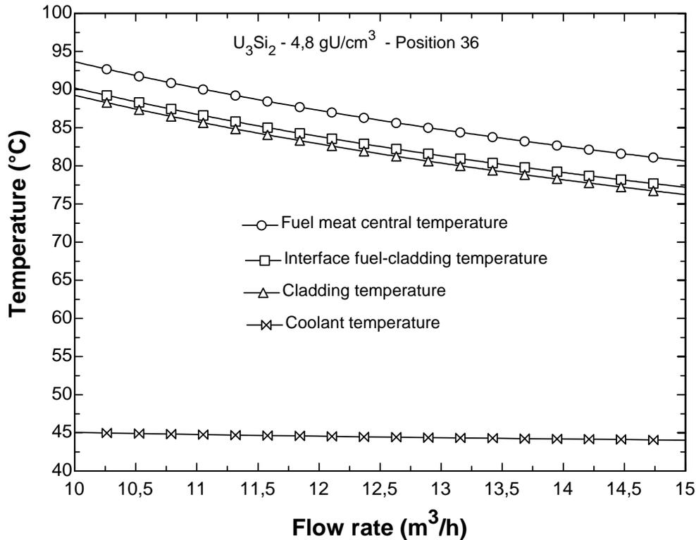
**Figure 4. Fuel miniplate and coolant calculated temperatures versus MID coolant flow rate ( $U_3Si_2 - 4.8 \text{ gU/cm}^3$  - Position 36 of the matrix plate of IEA-R1 reactor).**
