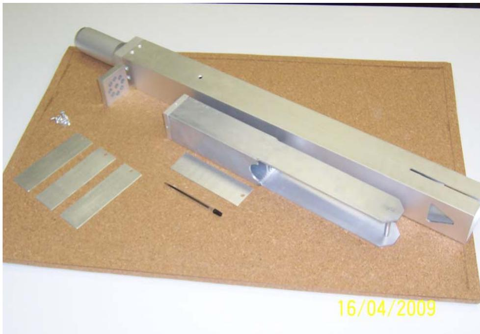
**Figure 1. – Miniplate Irradiation Device – MID.**
