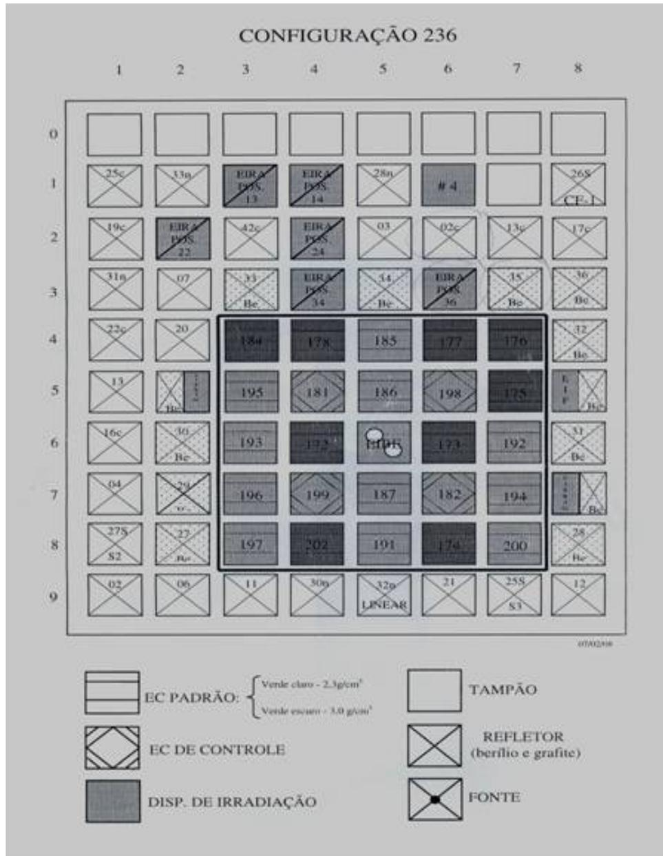
**Figura 3. – IEA-R1 reactor core.**
