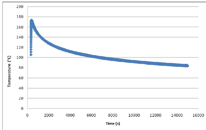
**Figura 8. Miniplates temperatures achieved after core draining in a postulated Primary Coolant Boundary Rupture accident.**
