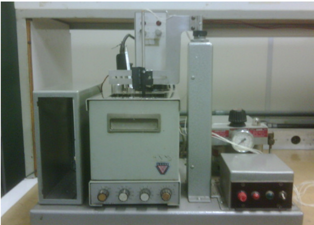
Figure 6. Plunge test experimental setup
