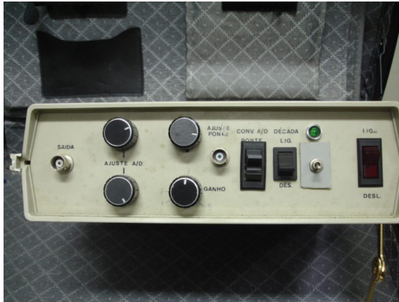
Figure 7. Loop current step response test equipment.
