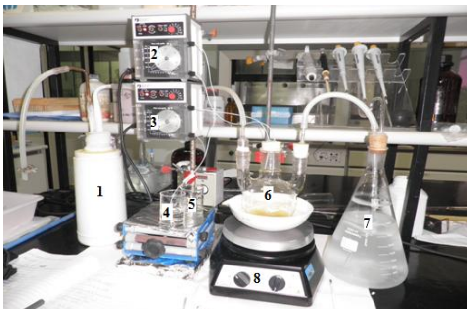
Figure 1: Experimental apparatus used in degradation experiments for a mixture of cationic and anionic resins. 1. Liquid nitrogen. 2 and 3. Peristaltic pumps. 4. Solution of hydrogen peroxide 50%. 5. Solution of catalyst. 6. Resin (anionic + cationic). 7. Solution of calcium hydroxide. 8. Magnetic stirrer (Model 753A).
