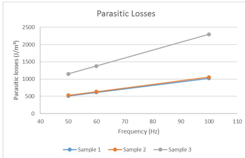
Fig. 4. Evolution of parasitic losses with increasing frequency for the three samples with different thicknesses. Data obtained from the Epstein test with induction of 1.5 T
