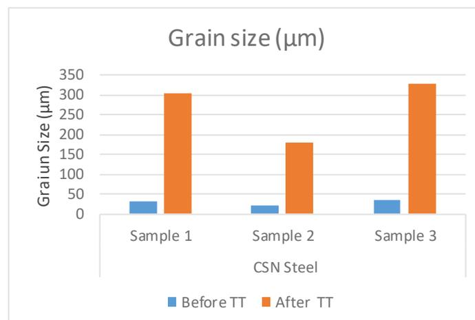
Fig. 2. Comparative graph showing the grain size of the samples before and after the heat treatment
