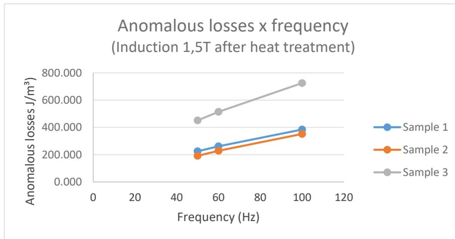
Fig.6. Relation of the anomalous losses after the heat treatment with the test frequency
