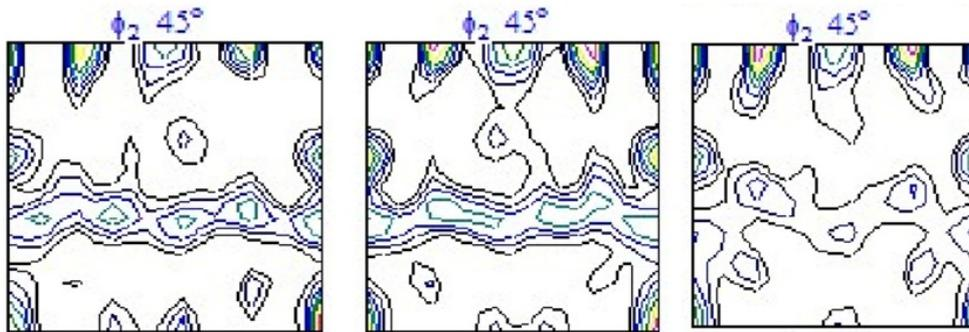
Fig. 3. ODF section  $\phi_1=0$  and  $\phi_2=45^\circ$  of samples 1, 2 and 3 respectively after the heat treatment
