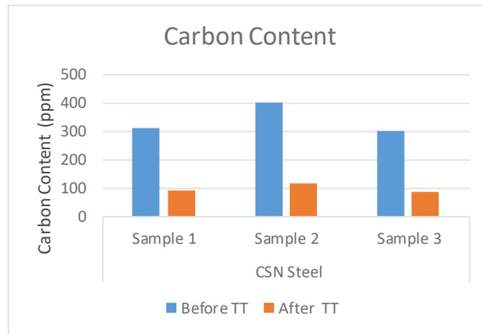
Fig. 1. Comparative graph of the variation of the carbon content of the samples analyzed before and after the heat treatment
