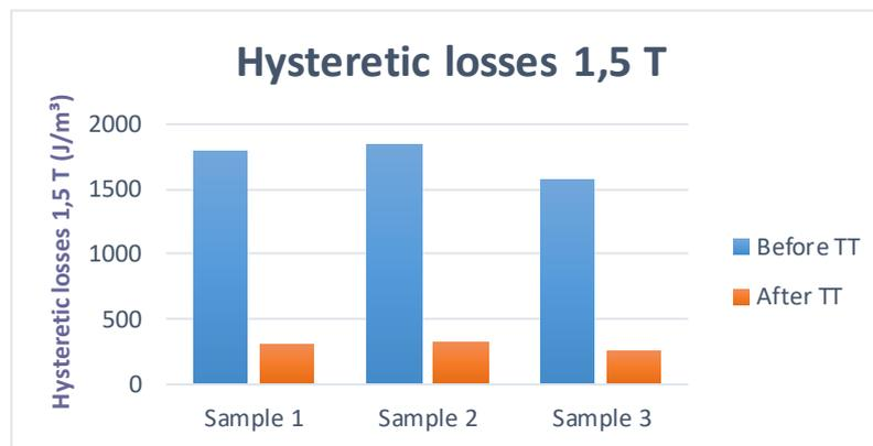
Fig. 5. Hysteretic losses before and after heat treatment of samples
