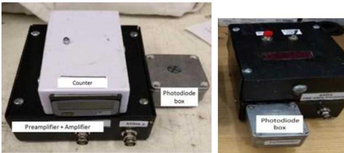
**Figure 3: Overview vision of the thermal neutron detector prototypes 1 (left) and 2 (right).**
