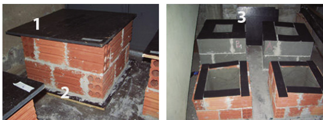
Fig. 1. Different views of test chambers built from concrete blocks and clay (red) bricks: 1—removable MDF cap, 2—bottom MDF fiberboard, 3—rubber strips used for airtightness of the internal volume of test chamber. (For interpretation of the references to color in this figure legend, the reader is referred to the web version of this article.)
