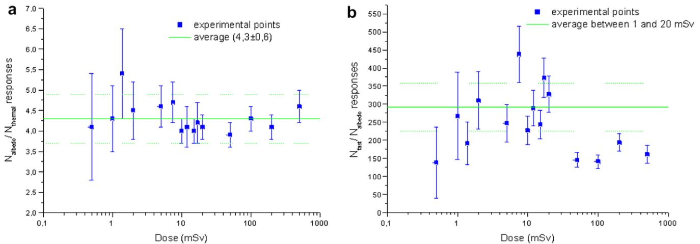
Fig. 3. Albedo to incident and albedo to fast neutron responses ratios.
