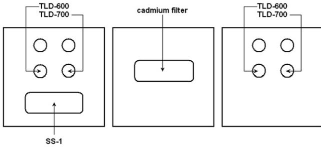
Fig. 1. Internal view of the neutron dosimeter.
