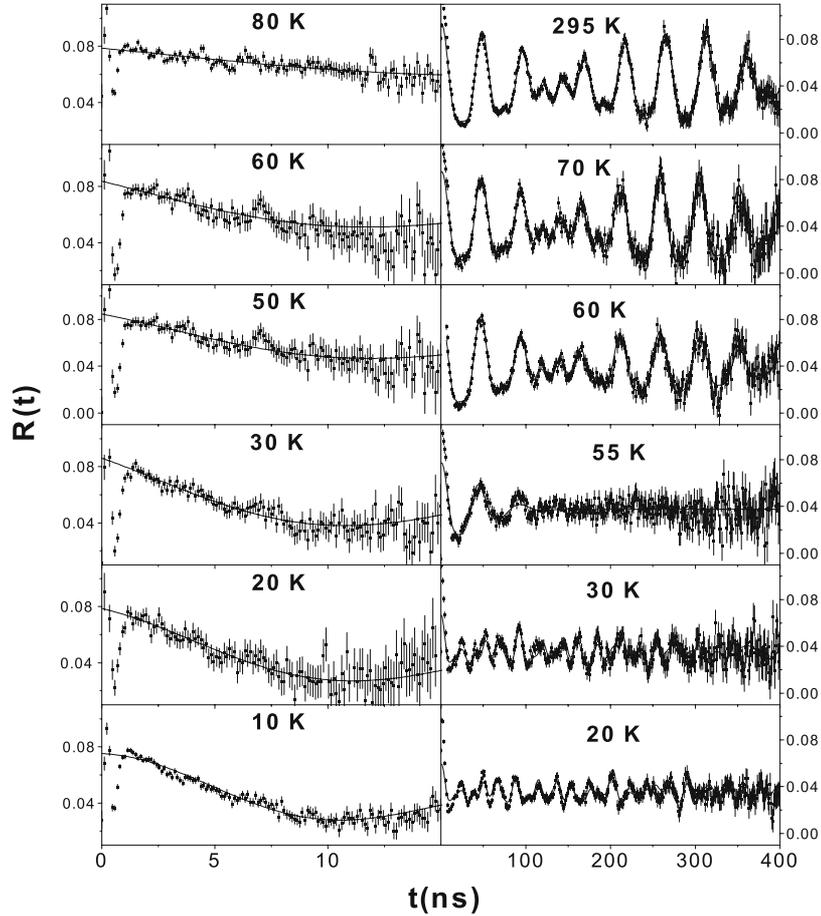
Figure 1. TDPAC spectra of the hyperfine interactions at Gd and In sites with  $^{140}\text{Ce}$  (left) and  $^{111}\text{Cd}$  (right) probes, respectively.
