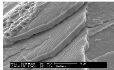
**Figure 2:** SEM image of a 12 h aged at 475 °C DSS. The fracture failure is brittle. Cleavage planes are clearly observed along the specimen and also a small area with dimples.
