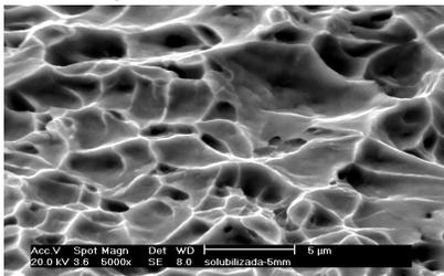
**Figure 1:** SEM image of a solution annealed DSS. The fracture is typically ductile and dimples are observed along the specimen.
