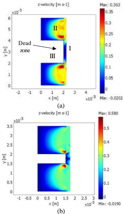
**Fig. 1:** z-velocity slice of (a) prototype A and (b) prototype B. The numbers I, II and III represent the position of the catalytic layer, channel and rib, respectively.
