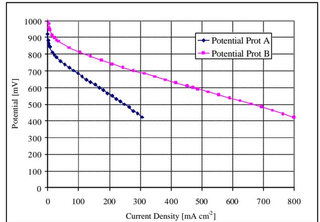
**Fig. 2:** Polarization curves of prototype A and B.
