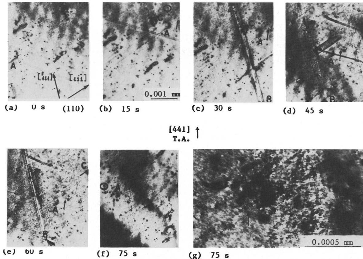
Fig. 1. In-situ deformation ( $2 \times 10^{-4}$  mm/s) of a Nb single crystal with [441] tensile axis during 900-keV HVEM observation.
