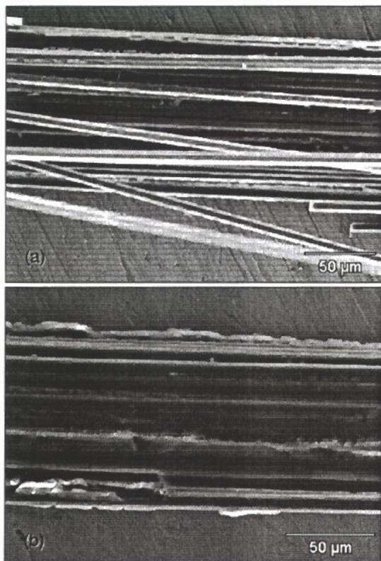
Fig.2 SEM micrographs of 12 k carbon fibers after breakage for (a) nonirradiated and (b) irradiated with 300 kGy samples.
