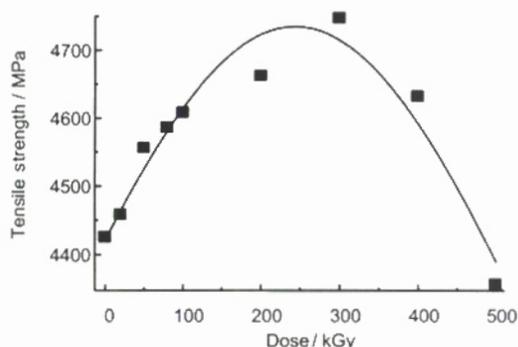
Fig.1 Tensile strength behavior of 12 k carbon fiber roving samples as a function of radiation dose applied.
