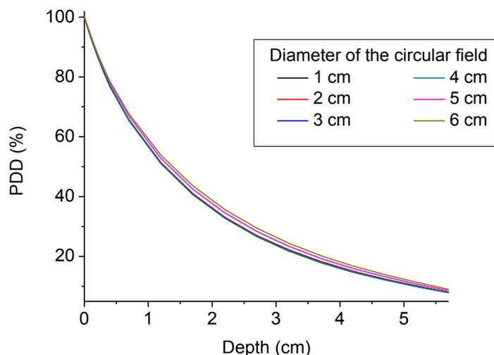
**Figure 6. Simulated PDD curves in function of the field size**
