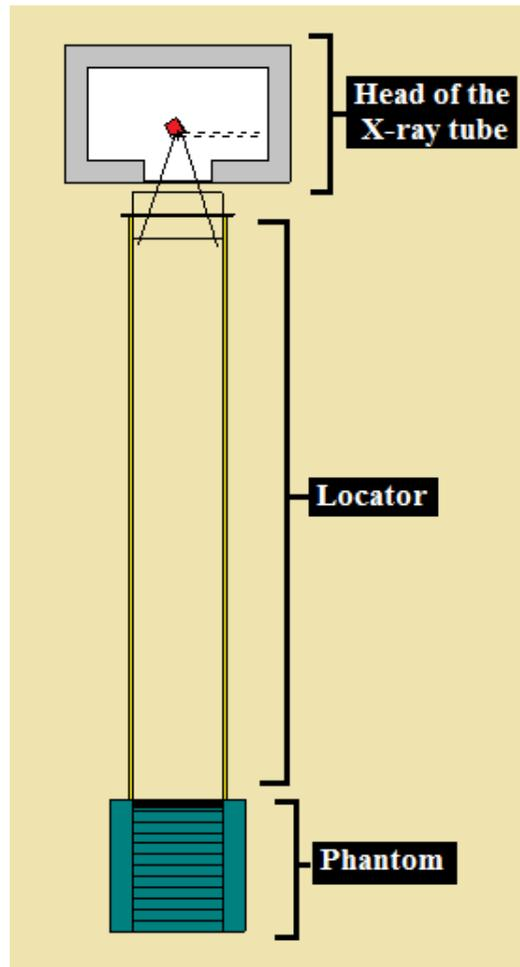
**Figure 5. System for PDD simulation**
