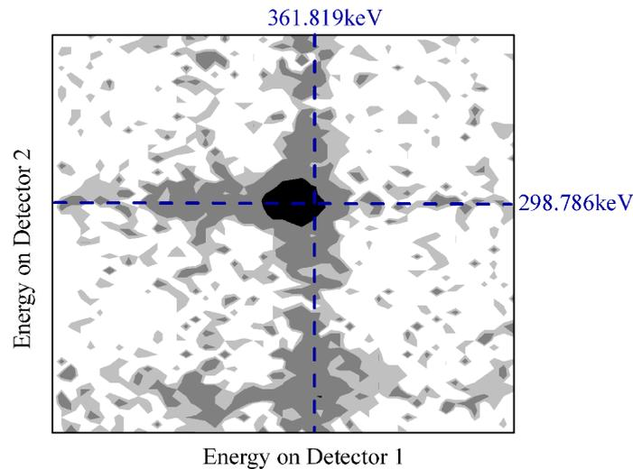
**Figure 3.** The bidimensional spectrum of the coincidence between the  $361.7\text{keV}$  and the  $298.8\text{keV}$  transitions.
