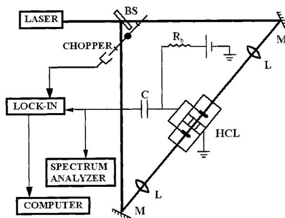
Fig. 1. Schematic diagram of intermodulated optogalvanic spectroscopy. The lamp construction diagram with electrical connections and a setup for noise measurement<sup>18</sup> are also included. BS, beam splitter; Ls, lenses; Ms, mirrors;  $R_b$ , ballast resistor; LOCK-IN, lock-in amplifier; C, capacitor.
