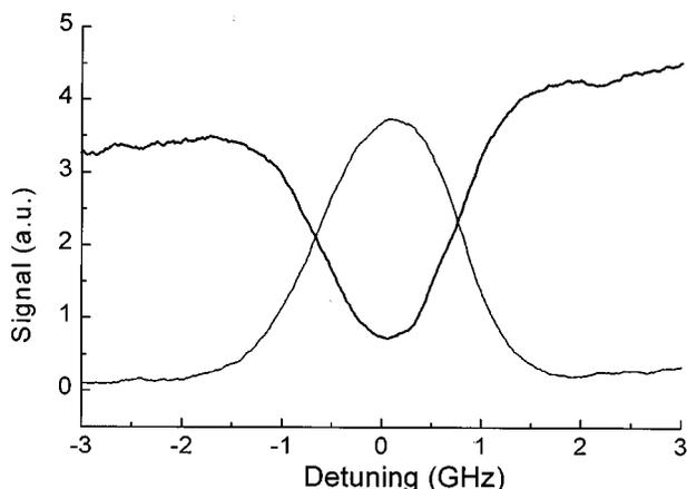
Fig. 4. Doppler-limited optogalvanic (lower curve) and optical absorption (upper curve) spectra of the calcium resonant transition at 423 nm, obtained at  $I = 30 \text{ mA}$ .
