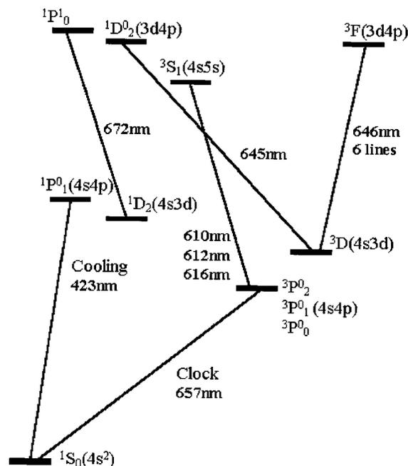
Fig. 2. Simplified level diagram of CaI.
