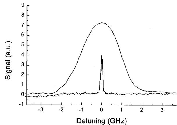
Fig. 3. Spectra of the CaI resonant transition at 423 nm, obtained simultaneously in the HCL (2.5 Torr Ca–Ar,  $I = 30$  mA) with optogalvanic detection (upper curve) and in an atomic beam with detection of fluorescence (lower curve).
