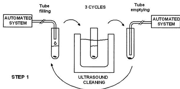
Fig. 2. Cleaning for external contamination (step 1).
