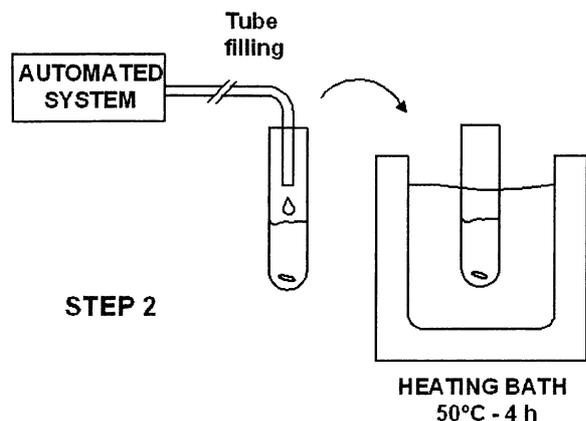
Fig. 3. Immersion in distilled water (step 2).
