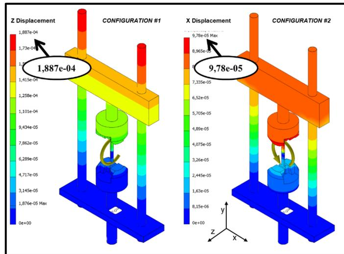
Figure 4 : Machine stiffness estimation results
