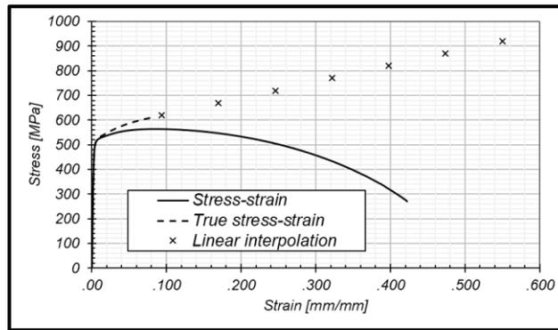
Figure 1 : API 5L x65MS stress-strain curve.
