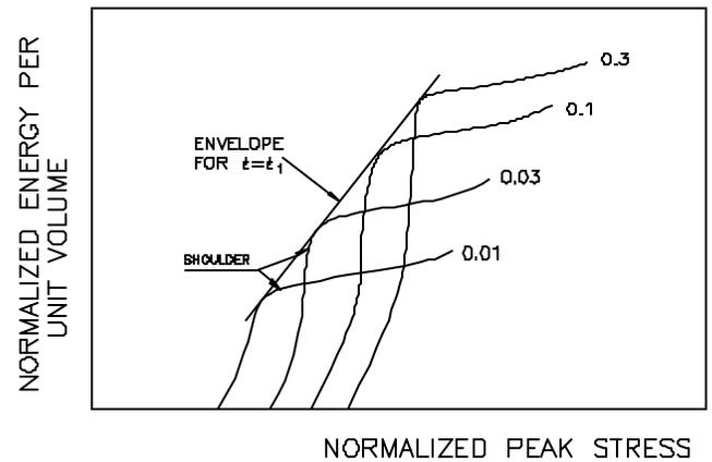
Figure 4(b) Specific absorbed energy plotted against stress  $\sigma_p$ , both parameters normalized by the solid polymer Young's modulus  $E_s$ .
