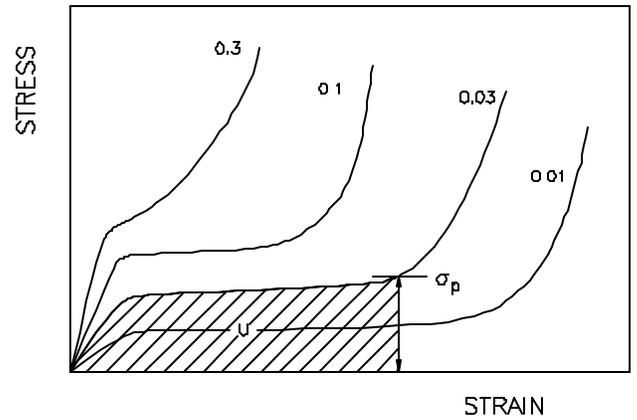
Figure 4(a). Stress-strain curves for various foam densities, measured at strain-rate  $\dot{\epsilon}_1$ . The area under each curve up to the stress  $\sigma_p$  is the absorbed energy per unit volume.
