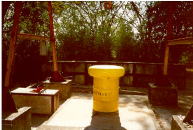
Figure 1(a) Type A package with shell type impact limiter tested at CDTN: before the drop test
