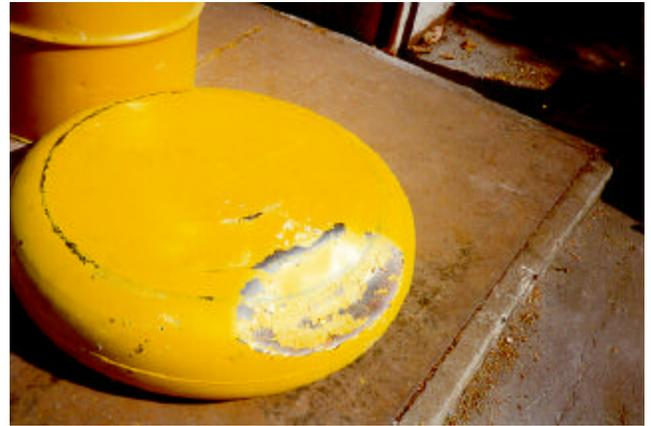
Figure 1(b) After the test, the damaged impact limiter removed from the package
