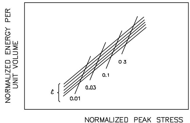
Figure 4(c) A family of envelope lines for different strain rates is plotted in the same axis as in (b), the points of same relative density (foam density/solid polymer density) connected by lines.
