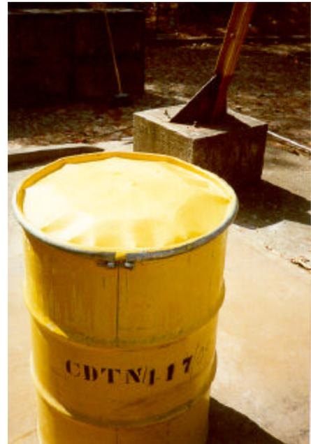
Figure 1(c) The package with some deformation at the lid
