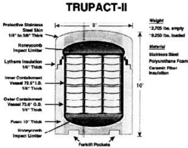
Figure 2. The TRUPACT-II, a package with impact limiter to transport transuranic wastes.
