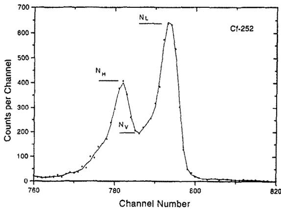
Fig. 6. Pulse height spectrum for  $^{252}\text{Cf}$  spontaneous fission fragments. The bias voltage amounts to 36 V in order to warrant the photodiode saturation condition.
