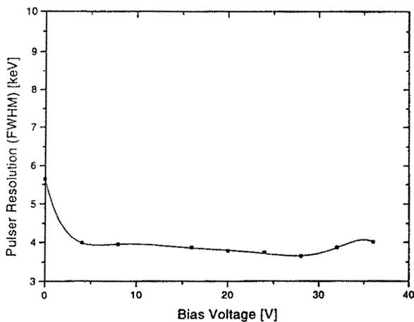
Fig. 2. Energy resolution (FWHM) of the pulse generator with the photodiode coupled to the preamplifier input as function of the bias voltage.
