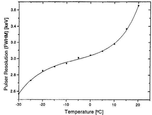
Fig. 3. Energy resolution (FWHM) of the pulse generator line, with the photodiode coupled to the preamplifier input, as function of the temperature. The bias voltage amounts to 28 V.
