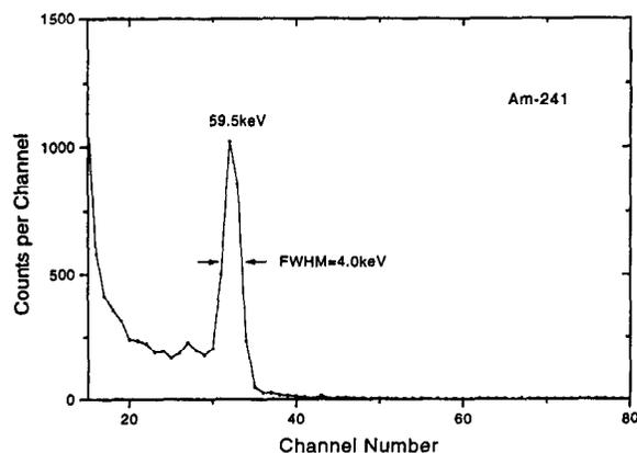
Fig. 10. Energy spectrum of  $^{241}\text{Am}$  59.55 keV  $\gamma$  line.
