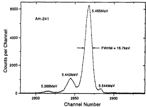
Fig. 5. Expanded view of the  $^{241}\text{Am}$  spectrum.
