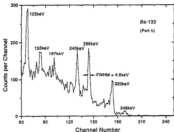
Fig. 9.  $^{133}\text{Ba}$  conversion electron spectrum (part b).
