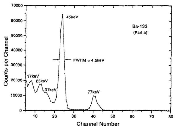
Fig. 8.  $^{133}\text{Ba}$  conversion electron spectrum (part a).
