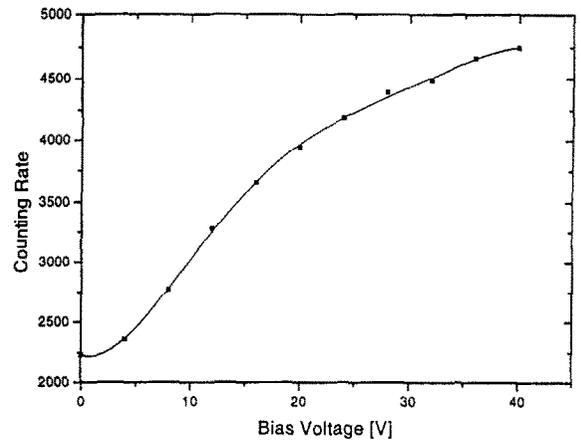
Fig. 7. The relative efficiency of the photodiode for internal conversion electrons as function of the polarization voltage.
