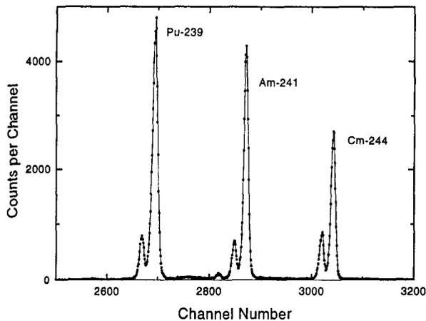
Fig. 4. Pulse height spectrum of  $^{239}\text{Pu}$ ,  $^{241}\text{Am}$  and  $^{244}\text{Cm}$  mixed source, recorded at a temperature of  $20^\circ\text{C}$  and a bias voltage of 28 V.
