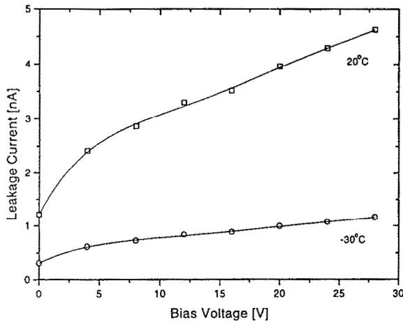
Fig. 1. The leakage current from the photodiode as function of the polarization voltage at 20 and  $-30^{\circ}\text{C}$ .
