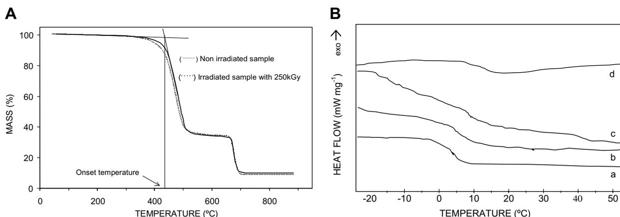
Fig. 2. (A) TG curves from non-irradiated sample (—) and from sample irradiated with 250 kGy (---); (B) DSC curves from: (a) non-irradiated sample, and samples after EB irradiation processing with different doses of (b) 75 kGy, (c) 150 kGy and (d) 250 kGy.
