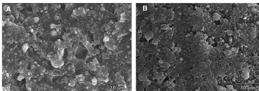
Fig. 3. SEM micrographs of fractured surfaces from: (A) non-irradiated sample and (B) sample after EB irradiation processing up to 250 kGy.
