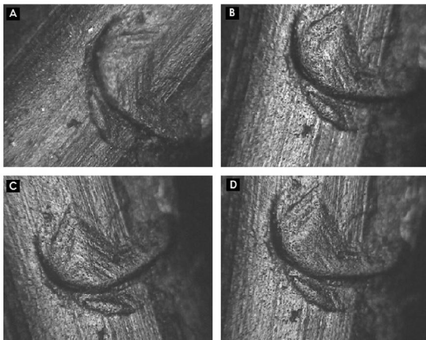
Fig. 4. Optical micrographs of the same O-ring surface defect: (A) non-irradiated sample and the same sample after irradiation processing up to doses of (B) 50 kGy, (C) 250 kGy and (D) 500 kGy.
