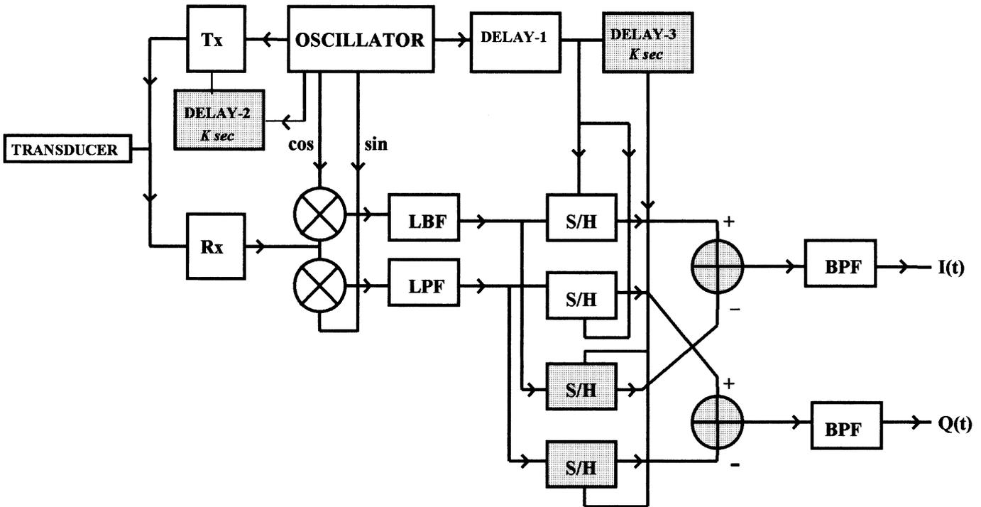
Fig. 4. Block diagram of a nonuniformly sampled directional PDUV. Tx stands for the transmitter amplifier, Rx is the receiver amplifier, LPF is a low-pass filter, BPF is a bandpass filter, and S/H are sample-and-hold devices.  $I(t)$  and  $Q(t)$  are in-phase and quadrature Doppler signals, respectively.
