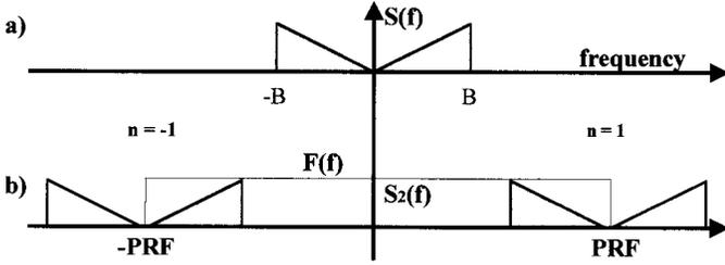
Fig. 2. (a) Spectrum of a low-pass signal; (b) spectrum of the low-pass signal of (a) second-order sampled: the replica at the origin is suppressed.  $F(f)$  is an ideal filter, used to select the lower bands of the replicas at  $n = \pm 1$ .
