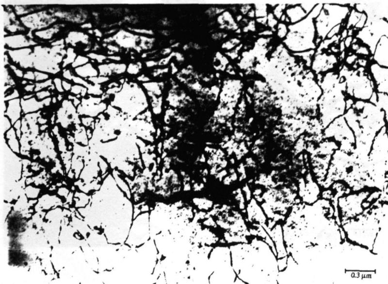
**Fig.115** Dislocation structure of a tensile tested specimen, 28% series, showing some dislocation debris. **B** [001].
