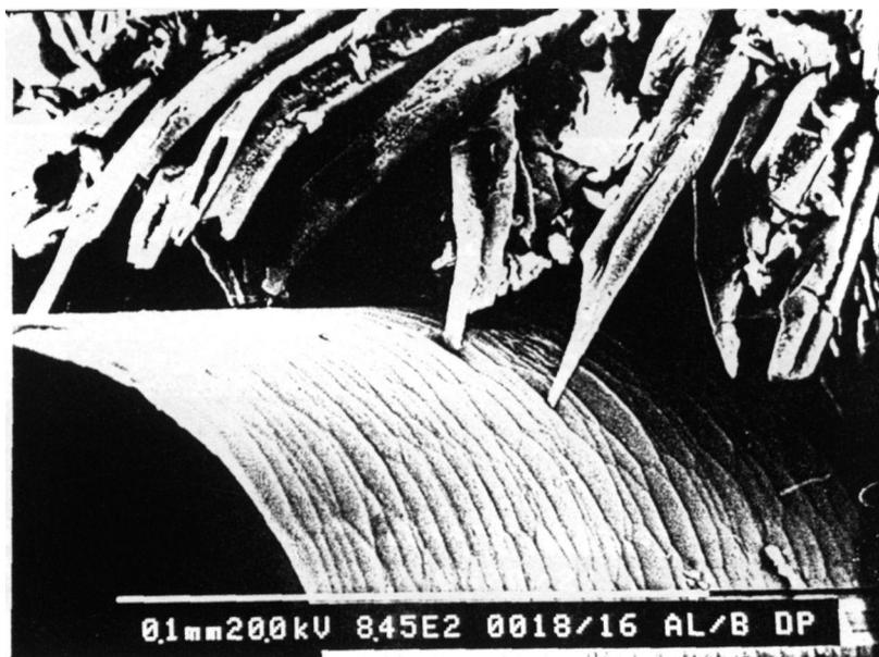
Fig.47 SEM micrograph of deep etched composite material series 28% showing a fibre and a complex particle network.
