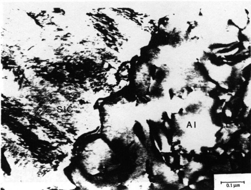
**Fig.60** TEM micrograph of interface aluminium/SiC for series 28% material. The micrograph shows the SiC coating (SiC) and the aluminium matrix with dislocations in contrast (Al). B<sub>Al</sub> [011].
