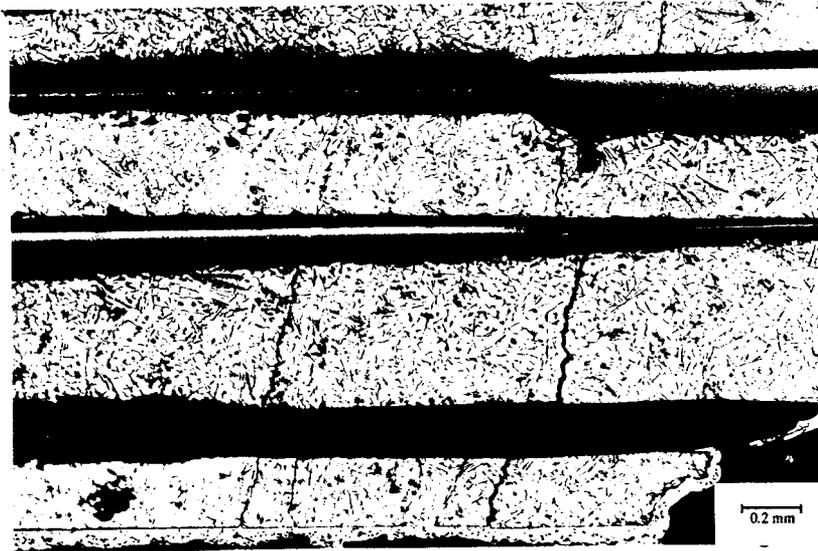
**Fig.108** Optical micrograph of a longitudinal section of a 28% series specimen fatigue tested, showing several matrix cracks. The fibres were usually kept intact. Some pieces of fibres were plucked out during the specimen preparation.
