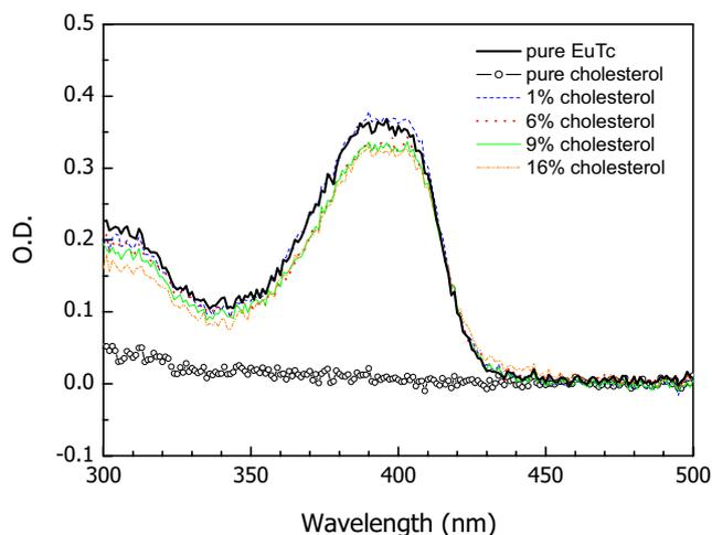
**Fig. 1** Absorption spectra for cholesterol, EuTc and EuTc + cholesterol solutions. The absorption spectrum of the EuTc solution shows weak dependence with cholesterol addition
