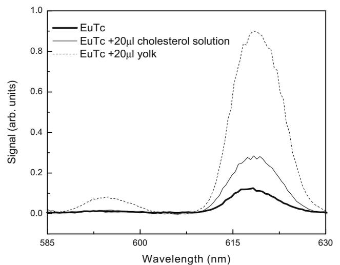
**Fig. 6** Europium emission band in solutions of EuTc, EuTc with 20  $\mu\text{l}$  of cholesterol and EuTc with 20  $\mu\text{l}$  of yolk egg obtained under excitation at 405 nm
