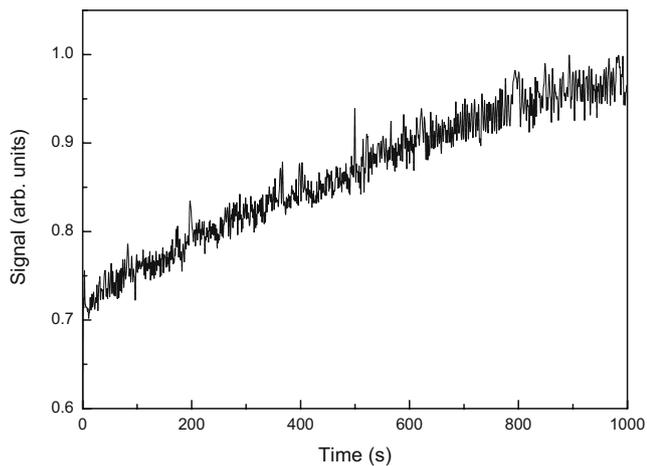
**Fig. 4** Dependence of the of 618 nm emission intensity with the time showing that stabilization occurs after 1,000 s
