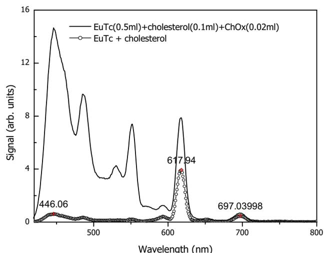
**Fig. 2** Emission spectra of EuTc/cholesterol (circles) and EuTc/cholesterol in the presence of cholesterol oxidase (line) obtained under excitation at 405 nm
