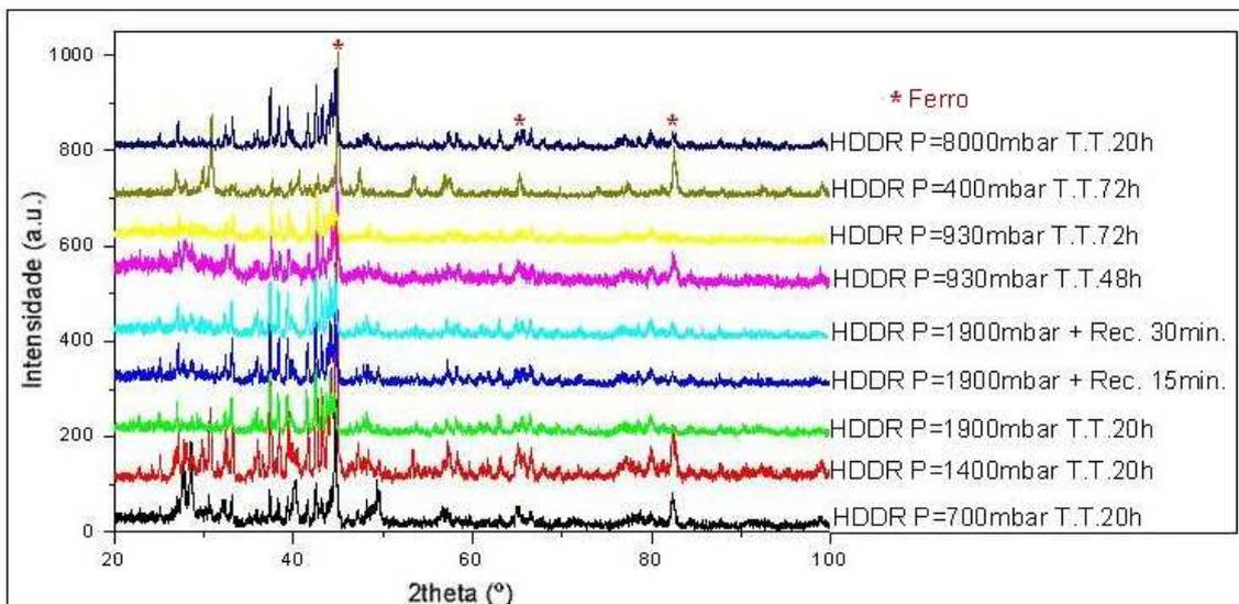
**Fig. 2**- X-ray diffraction patterns of the  $\text{Pr}_{12}\text{Fe}_{65.9}\text{Co}_{16}\text{B}_6\text{Nb}_{0.1}$  HDDR powders.
