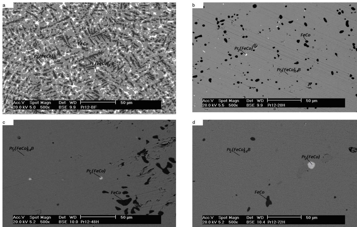
**Fig. 4-** SEM microstructures of the  $\text{Pr}_{12}\text{Fe}_{65.9}\text{Co}_{16}\text{B}_6\text{Nb}_{0.1}$  alloy; (a) cast alloy, treated for (b) 20 h, (c) 48 h and (d) 72 h.
