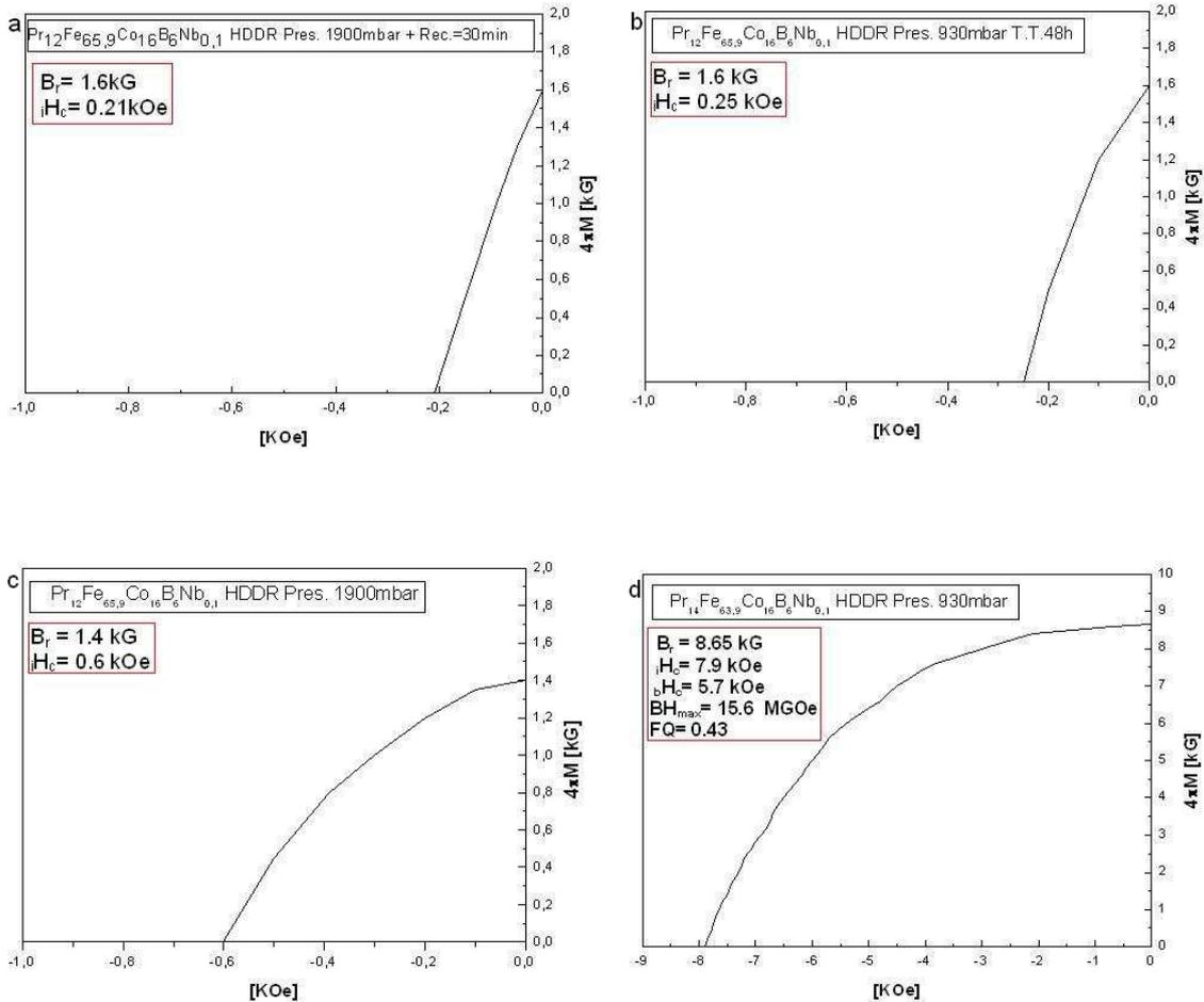
**Fig. 1** - (a, b and c) Demagnetization curves of the  $\text{Pr}_{12}\text{Fe}_{65.9}\text{Co}_{16}\text{B}_6\text{Nb}_{0.1}$  bonded magnets with best values of  $B_r$  and  $H_c$  values, (d) demagnetization curve of the standard  $\text{Pr}_{14}\text{Fe}_{63.9}\text{Co}_{16}\text{B}_6\text{Nb}_{0.1}$  magnet.
