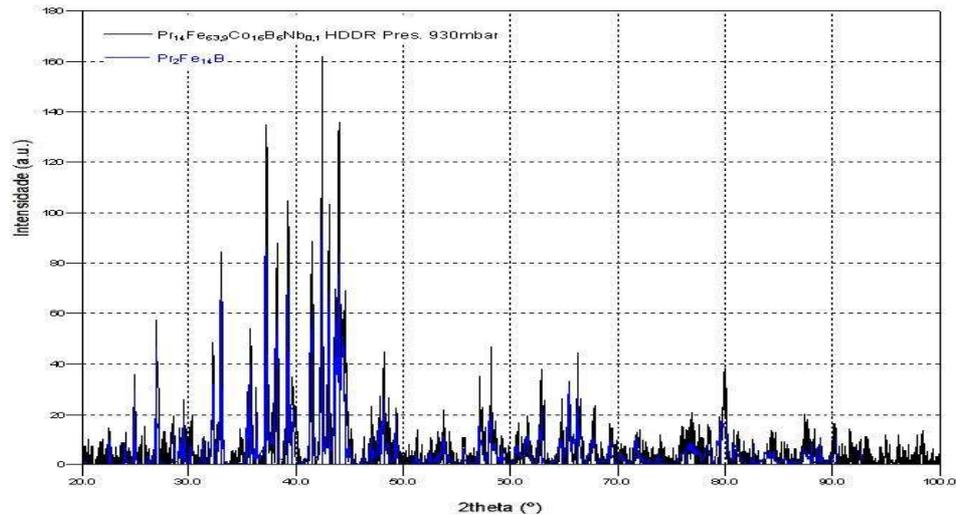
**Fig. 3-** X-ray diffraction patterns of  $\text{Pr}_{14}\text{Fe}_{63.9}\text{Co}_{16}\text{B}_6\text{Nb}_{0.1}$  powders.
