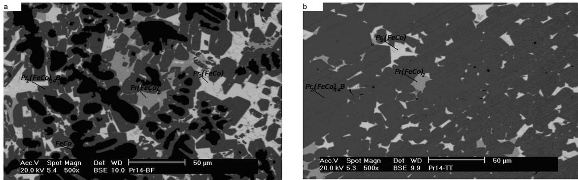
**Fig. 5-** SEM microstructures of the  $\text{Pr}_{14}\text{Fe}_{63.9}\text{Co}_{16}\text{B}_6\text{Nb}_{0.1}$  alloy; (a) cast alloy and (b) with a heat treatment of 20 h.
