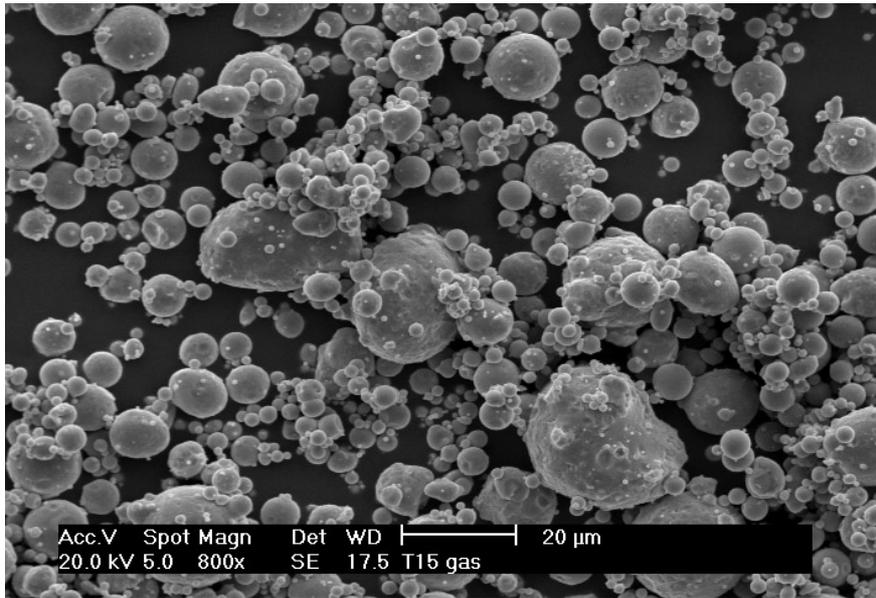
Fig.1 – Scanning electron micrograph showing the spherical morphology of the particles of the AISI T15 powders.
