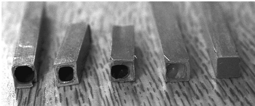
Fig. 4 - Irregular fulfilling of the mold indicating a very high temperature of injection.
