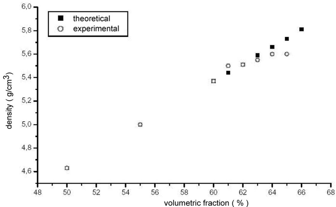
Fig. 2 – Critical load determination of the AISI T15 steel powder for the binder system used in the work.
