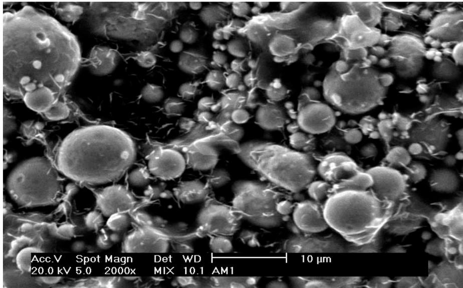
Fig. 5 - SEM micrograph of green part fracture showing the uniformity of the dispersal of the binder PW/PE/AS .
