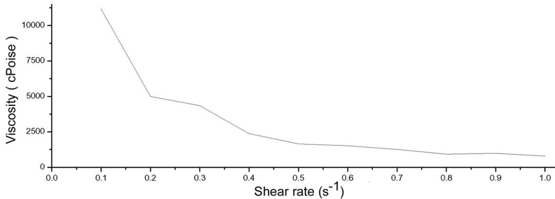
Fig. 3 - Rheological pseudo-plastic behavior of the feedstock remaining for a long period.
