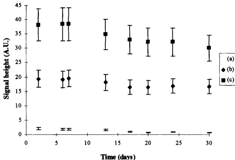
Fig. 3. ESR signal decay: Non irradiated (a), 3.5 kGy (b) and 7.0 kGy (c)
