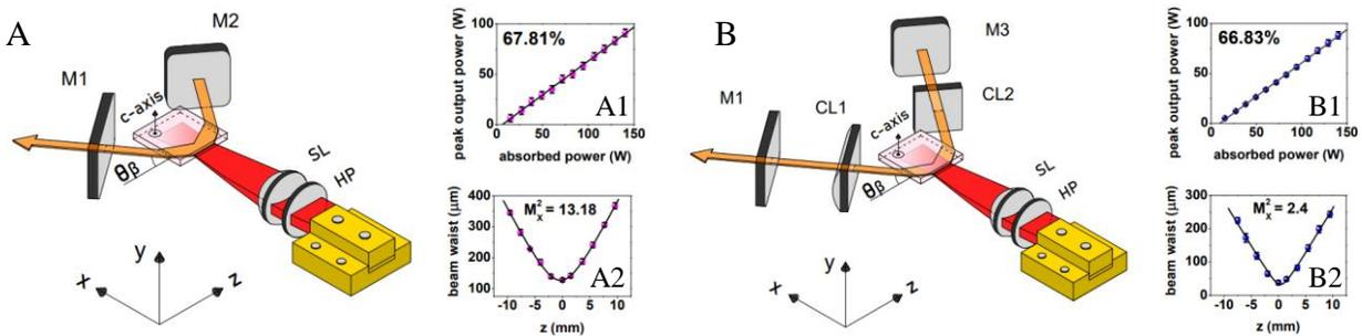
Fig. 1. A: Plane-concave resonator. A1: peak output power vs absorbed power of the PC resonator. A2: PC beam waist curve fit. B: Plane-plane resonator. B1: peak output power vs absorbed power of the PP resonator. B2: PP beam waist curve fit
