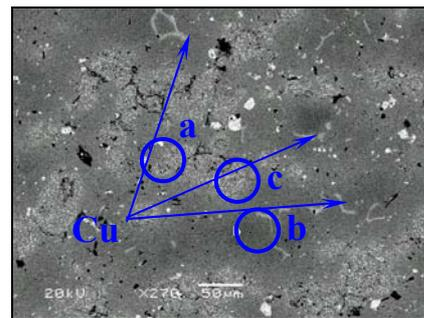
Figure 6 – SEM micrography of alloy 1 in the as sintered and heat treated condition.
