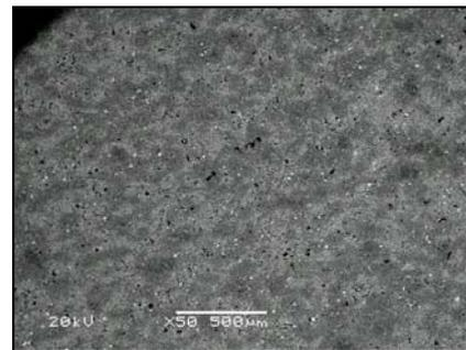
Figure 2 – SEM micrography of alloy 1 in the as sintered and heat treated condition.
