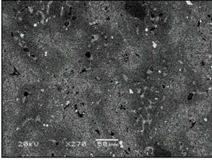
Figure 8 – SEM micrograph of alloy 2 in the as sintered condition.
