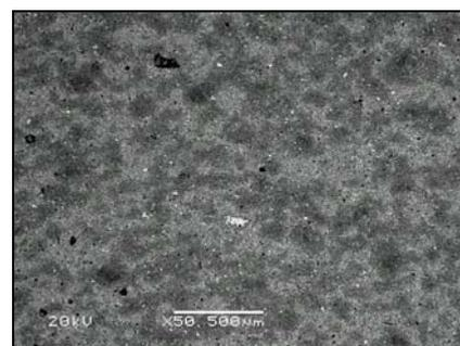
Figure 4 – SEM micrography of alloy 2 in the as sintered and heat treated condition.
