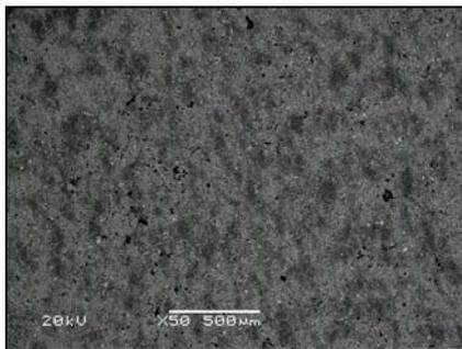
Figure 1 – SEM micrography of alloy 1 in the as sintered condition.
