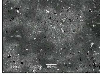
Figure 9 – SEM micrograph of alloy 2 in the as sintered and heat treated condition.
