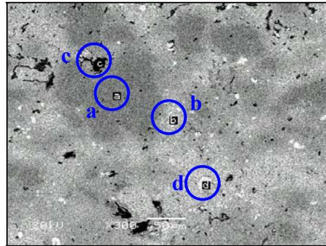
Figure 10– SEM micrograph of alloy 2 in the as heat-treated condition.
