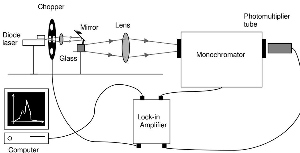
FIGURE 1. System for emission measurements.
