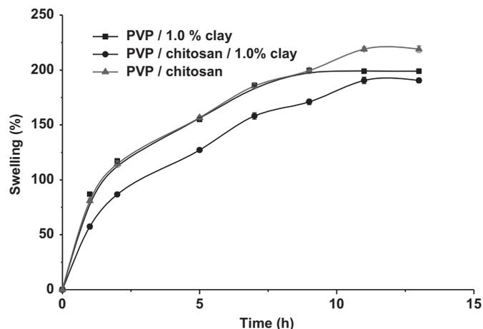
Fig. 1. Swelling curves of hydrogels PVP/clay, PVP/chitosan/clay and PVP/chitosan, obtained by gamma irradiation at 25 kGy dose.
