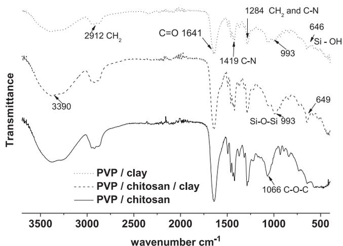
Fig. 6. FTIR spectra of PVP/clay, PVP/chitosan/clay and PVP/chitosan hydrogels, obtained by gamma irradiation, dose 25 kGy.
