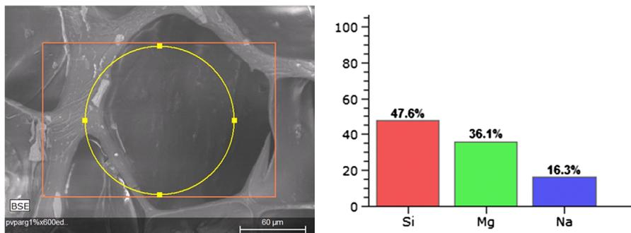
Fig. 4. Microscopy and EDS of lyophilized hydrogel PVP/1% clay obtained by gamma irradiation at 25 kGy dose.
