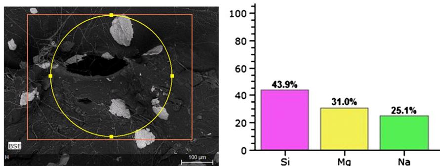
Fig. 5. Microscopy and EDS of lyophilized hydrogel PVP/chitosan/1% clay obtained by gamma irradiation at 25 kGy dose.
