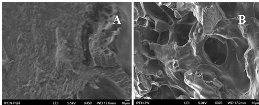
Fig. 3. SEM images (A) of dried PVP/chitosan hydrogel and (B) dried PVP/chitosan hydrogel with 1.0% of clay laponite RD obtained by gamma irradiation at 25 kGy dose.
