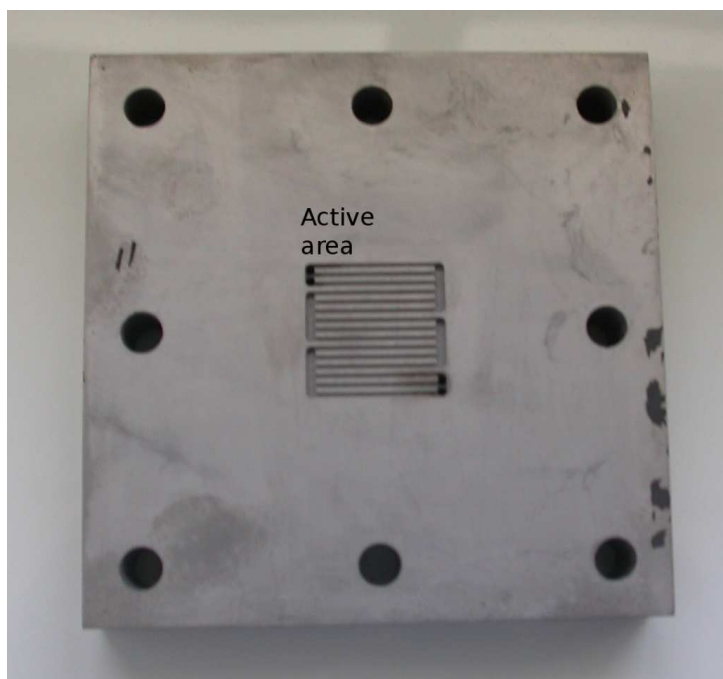
Figure 4: Graphite plate coated with nickel
