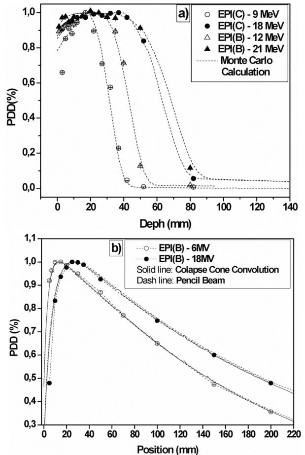
Fig. 4. PDD profiles in PMMA under irradiation with: (a) 9, 12, 18 and 21 MeV electron beams; (b) 6 and 18 MV photon beams. Monte Carlo (lines), Collapse Cone Convolution (solid line) and Pencil Beam (dash line) calculations are presented for comparison. Experimental uncertainties are smaller than the symbols size.
