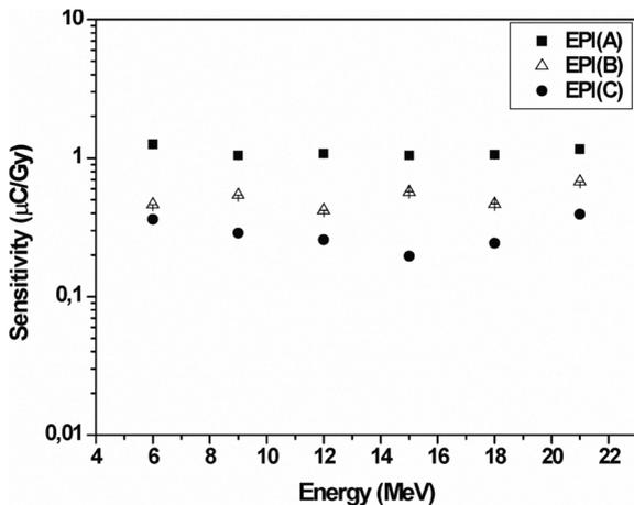
Fig. 3. Charge sensitivities of EPI diodes as a function of the electron beam energy. Experimental uncertainties are smaller than the symbols size.
