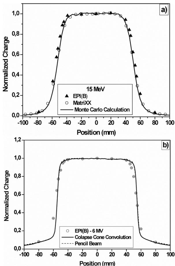
Figure 5: TDP measurements performed in PMMA with the EPI diodes for: (a) 15 MeV electron beam irradiation; (b) 6 MV photon beam irradiation. For comparison, Collapse Cone Convolution (solid line) and Pencil Beam (dash line) calculations are presented. Experimental uncertainties are smaller than the symbols size.
