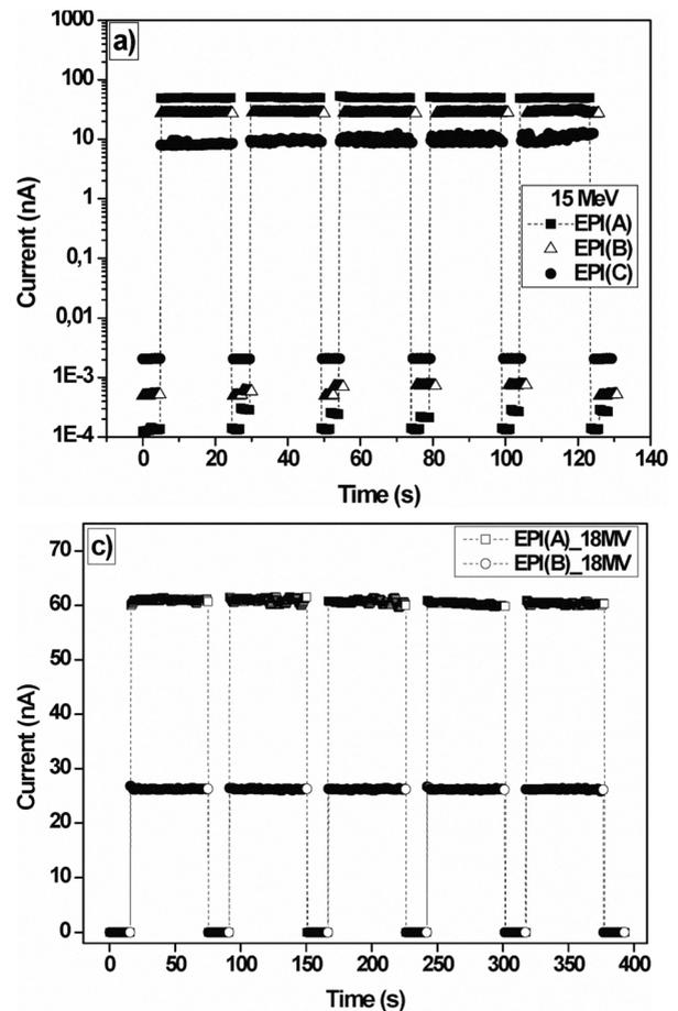
Fig. 1. Five signals consecutively registered with the diodes under irradiation with: (a) 15 MeV electron beam irradiation at 5.0 cGy/s dose rate; (b) 18 MV photon beam at 3.70 cGy/s dose rate.
