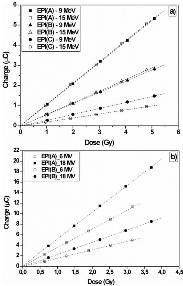
Fig. 2. Dose-Response curves of EPI diodes for: (a) 9 and 15 MeV electron beam energies; (b) 6 and 18 MV photon beam energies. Experimental uncertainties are smaller than the symbols size in both figures.
