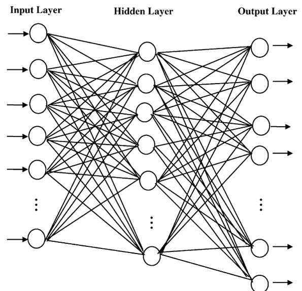
Fig. 1. Multilayer Perceptron 10-50-52 used for unfolding neutron spectra.
