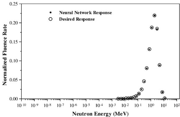
Fig. 4. Comparison between Neural Network output and the expected neutron spectrum.
