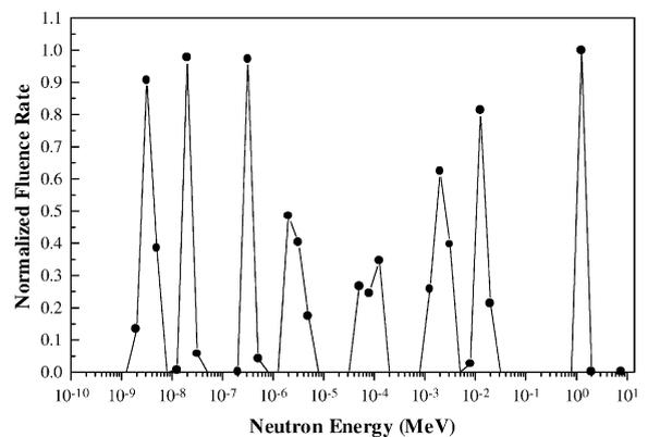
Fig. 3. Neural Network output spectrum for eight different monoenergetic neutron beams. The input data corresponding to the Bonner Sphere counting rates were allowed to spread, in order to simulate a Normal distribution with 5% relative standard deviation.
