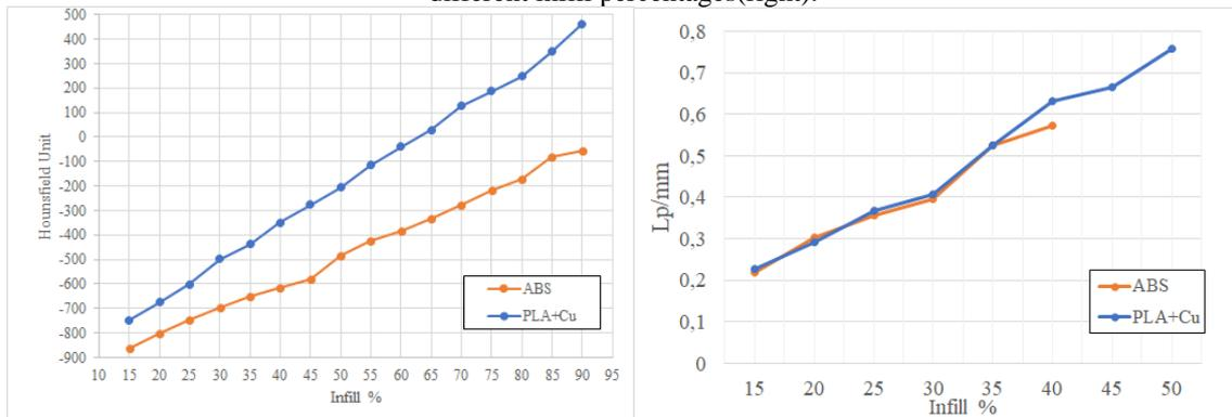
**Figure 2:** measurements on 15% to 50% infill samples.PLA+Cu (left) and ABS (right)
