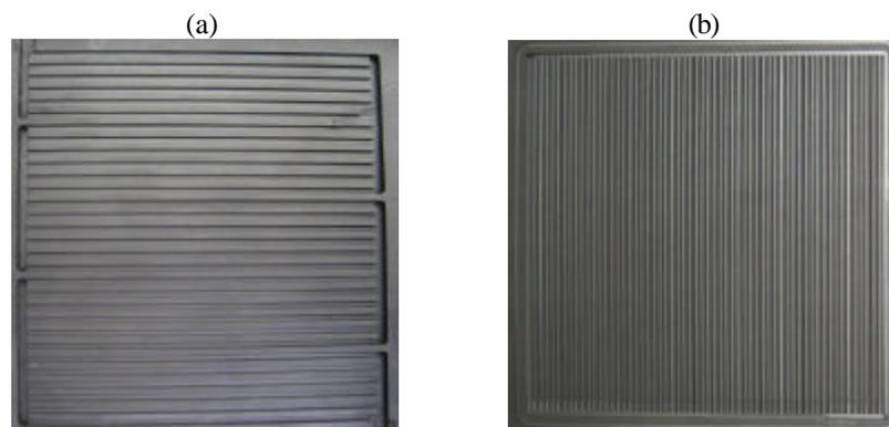
**Figure 1:** Flow field channels from prototype 1 (a) and prototype 2 (b).
