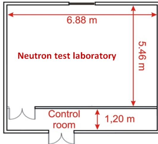
**Figure 2: Simplified floor plan of the Neutron Test Laboratory.**
