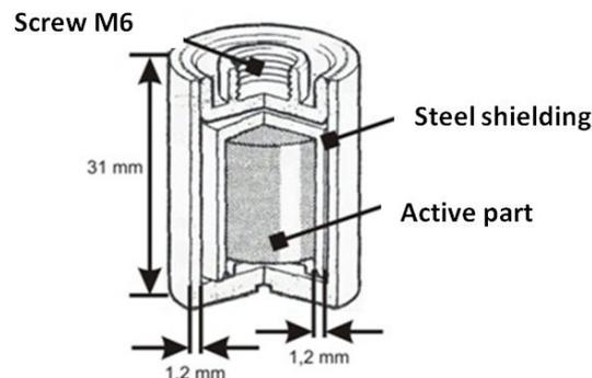
Figure1: Neutron source of  $^{241}\text{Am}(\text{Be})$  at the Neutron Test Laboratory (LTN) .
