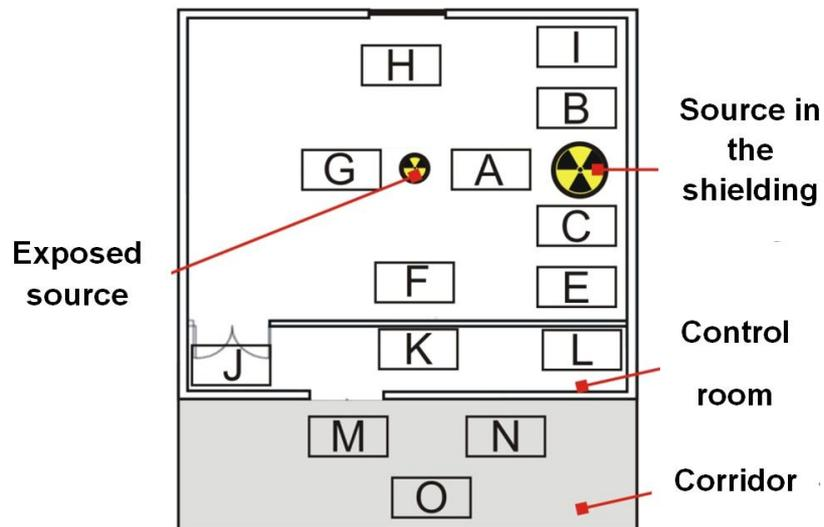
**Figure 3: Floor plan of LTN, identifying the points for the radiometric survey. The measuring point D is located at the top of the source shielding, and can not be seen in this figure.**
