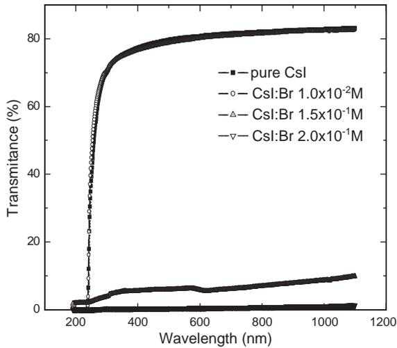
Fig. 1. Transmittance curves of CsI pure and doped with  $10^{-2}$ ,  $1.5 \times 10^{-1}$  and  $2.0 \times 10^{-1}$  mol.
