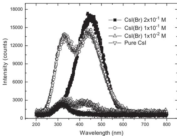
Fig. 2. Luminescence spectra (b) of CsI pure and doped with  $10^{-2}$ ,  $10^{-1}$  and 1 mol.
