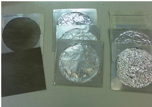
**Figure 1: Filters used in this study. Molybdenum (left) and Aluminum.**
