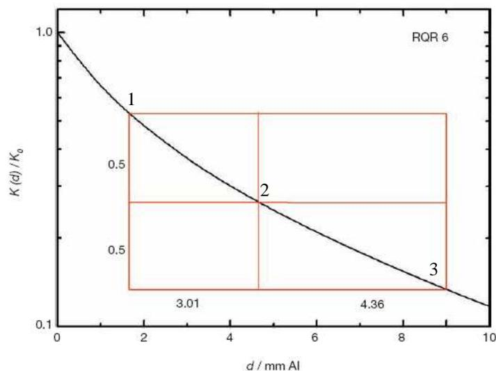
**Figure 4: Example of the attenuation curve expressed as the ratio of the air kerma,  $K(d)$ , behind a filtration of thickness,  $d$ , to the air kerma,  $K_0$ , of the unattenuated beam. (Withdrawal from the TRS-457, page 72)**
