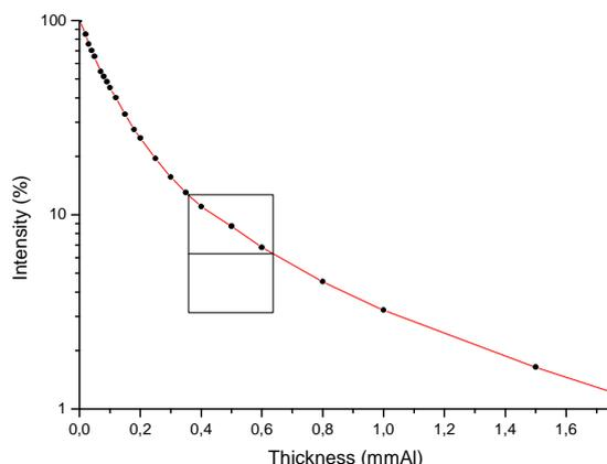
**Figure 6: Attenuation curve for RQR-M 1, using the HVL value given by the IEC 61267[1]**
