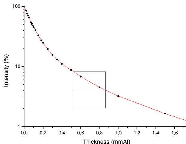
**Figure 5: Attenuation curve for RQR-M 1, based on the TRS-457**
