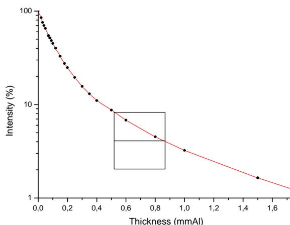
**Figure 7: Attenuation curve for RQR-M 1, using the HVL value given by PTB**
