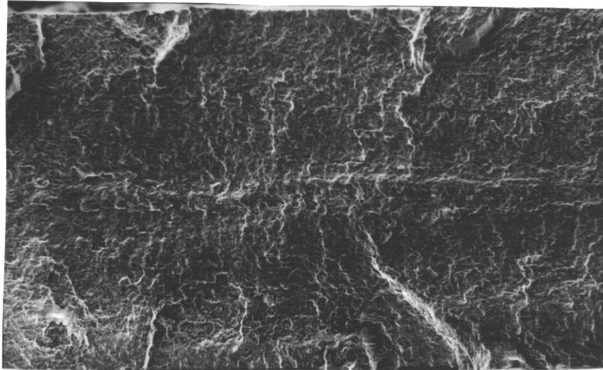
FIG. 1 - Fracture surface of DPS tested at 400 MPa. This view shows the stretched zone near at center.
