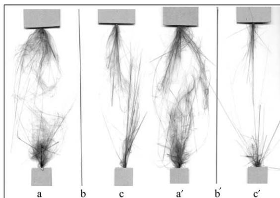
Fig. 1. 6k carbon fiber test specimens: non-irradiated, after breakage (a), before tensile test (b), and irradiated with 300 kGy, after breakage (c). 12k carbon fiber test specimens: non-irradiated, after breakage (a'), before tensile test (b'), and irradiated with 300 kGy, after breakage (c').
