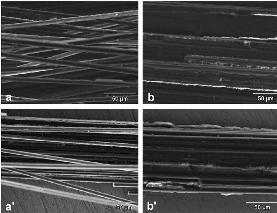
Fig. 2. SEM micrographs of 6k and 12k carbon fibers after breakage for non-irradiated (a, a') and irradiated (b, b') samples, respectively.
