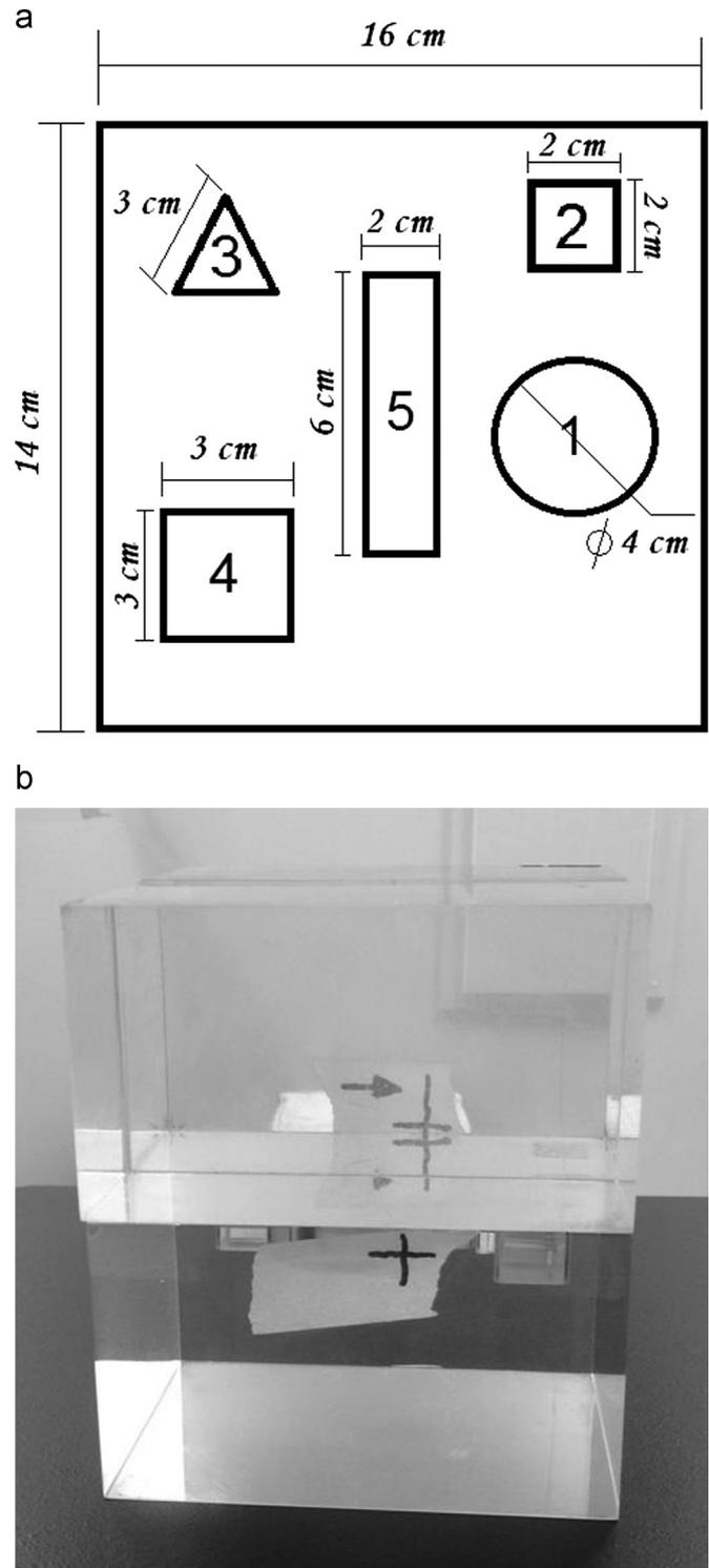
Fig. 1. (a) Project of PMMA phantom containing five cavities and (b) PMMA block used upon phantom with microdosimeters positioned to irradiation.
