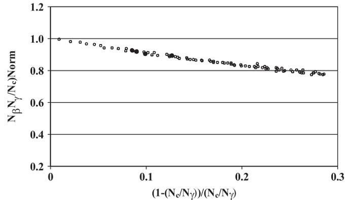
Fig. 1. Normalized Monte Carlo simulation of predicted  $N_{\beta}N_{\gamma}/N_c$  as a function of efficiency parameter  $(1 - N_d/N_{\gamma})/(N_d/N_{\gamma})$  for  $^{35}\text{S}$  (open circles). Black circles correspond to normalized experimental data.
