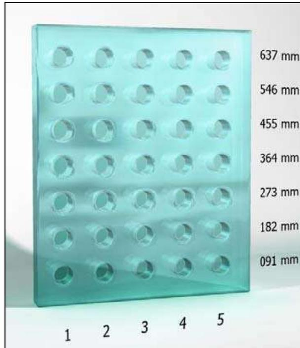
**Figure 2: Illustration of the Lucite plate and the positions of the gold foils on it.**
