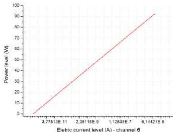
**Figure 6 : Calibration straight line to nuclear power channel 6 for cylindrical configuration.**
