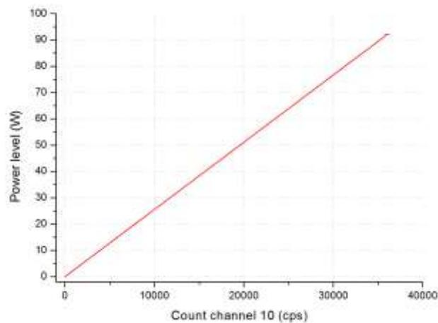
**Figure 7 : Calibration straight line to nuclear power channel 6 and count in channel 10 for cylindrical configuration.**
