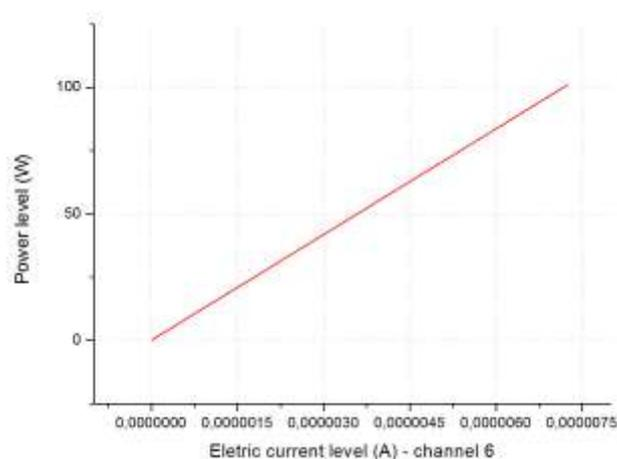
**Figure 4 : Calibration straight line to nuclear power channel 6 for rectangular configuration.**
