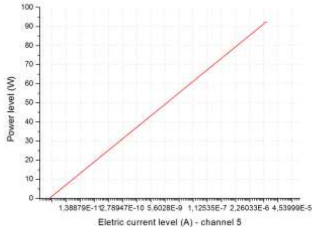
**Figure 5 : Calibration straight line to nuclear power channel 5 for cylindrical configuration.**
