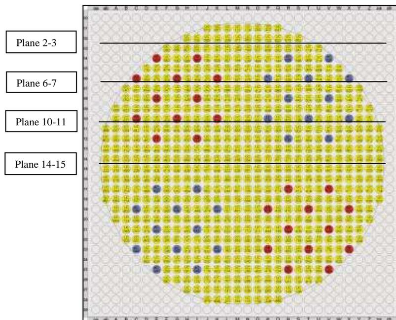
**Figure 1: Cylindrical Configuration of IPEN-MB/01 Reactor (28x28 fuel rods) and planes of irradiation - Superior view.**
