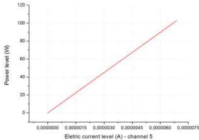
**Figure 3 : Calibration straight line to nuclear power channel 5 for rectangular configuration.**
