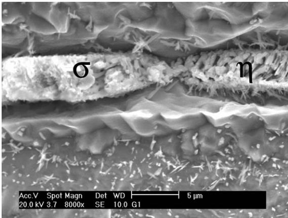
Fig. 7. Micrographs of the gauge length of the tested specimen (600 °C/70 MPa/85 000 h), showing precipitation of the sigma and Laves phases in delta ferrite, and intra-granular precipitation of the Laves phase. Deep etching with V2A-etchant. SEM. SE.
