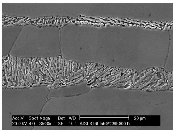
Fig. 4. Sigma ( $\sigma$ ) phase formation from delta ferrite islands after 85 000 h creep test at 550 °C. Etching: V2A-Beize. SEM. SE.
