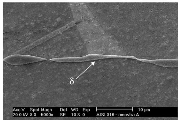
Fig. 2. Scanning electron micrograph (secondary electrons) of solution-annealed 316L(N) stainless steel, showing details of the delta ( $\delta$ ) ferrite phase. Etching: V2A-etchant.
