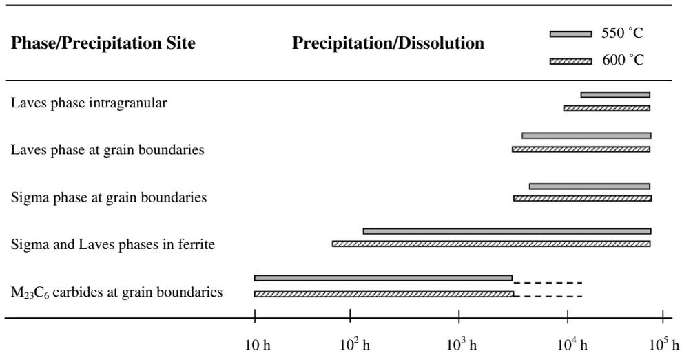
Fig. 3. Schematic diagram of phase reactions during ageing of AISI 316L(N) at 550 and 600 °C.
