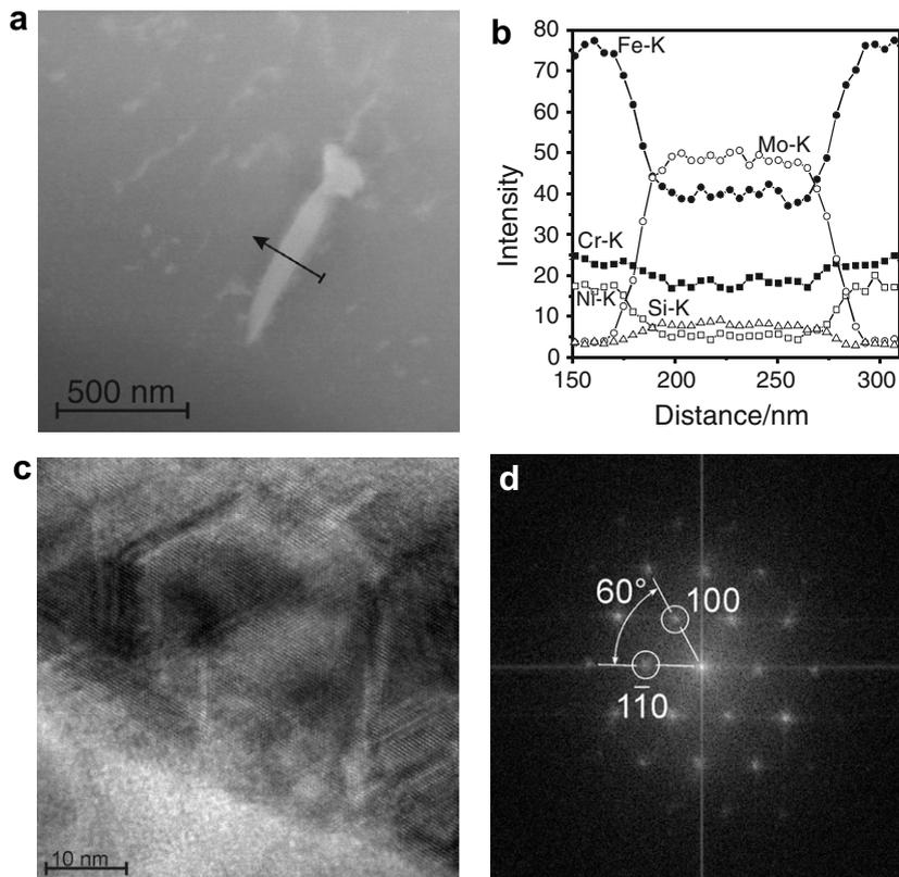
Fig. 9. TEM analysis of the Laves phase: (a) bright-field image; (b) Fe, Cr, Ni, Mo, and Si profiles along the arrow in (a); (c) high-resolution image of the Laves phase; (d) zone axis [00 1], hexagonal structure with  $a = 0.4745$  nm and  $c = 0.7734$  nm.
