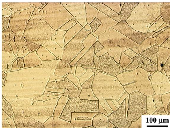
Fig. 1. Optical micrograph of solution-annealed 316L(N) stainless steel, revealing the presence of recrystallised grains and annealing twins. Etching: V2A-etchant.
