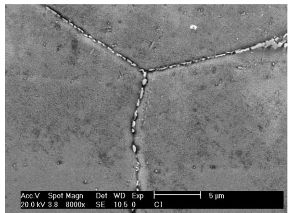
Fig. 5. Sigma ( $\sigma$ ) phase precipitation at austenite grain boundary and triple points after 85 000 h creep test at 550 °C. Etching: 5% HCl in ethanol. SEM. SE.
