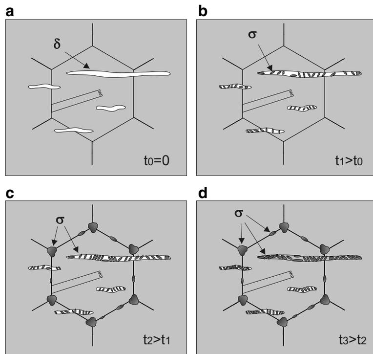
Fig. 6. Schematic presentation of sigma phase formation [25,26] in AISI 316L(N) at 550 and 600 °C.
