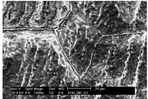
Fig. 8. Micrograph showing sigma phase precipitation at grain boundaries and intra-granular precipitation of the Laves phase after 85 000 h creep test. Deep etching with V2A-etchant. SEM. SE.
