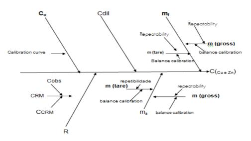
Figure 1. Cause-effect diagram of the sources of uncertainty associated with the measurement of Cu and Zn.
