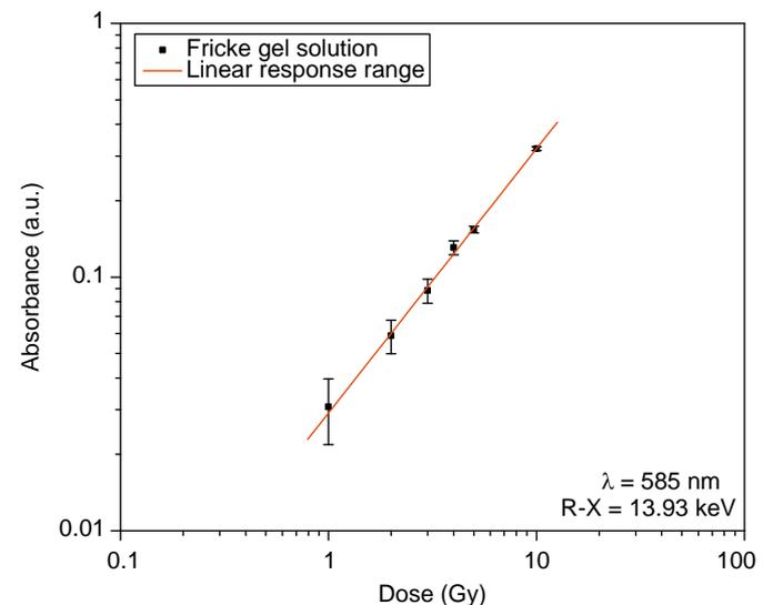
Fig. 7. Dose response curve of the Fricke gel solution to 13.93 keV X-rays.
