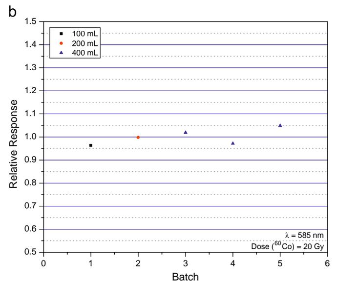
Fig. 4. Spectrophotometric response (relative to the mean value) reproducibility of the non-irradiated (a) and irradiated (b) Fricke gel solution for different solution batches.
