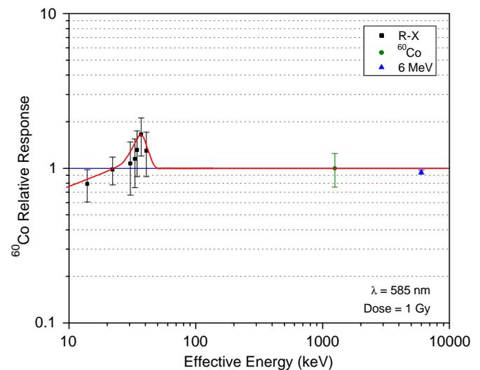
**Fig. 1.** Spectrophotometric energy dependent response of the Fricke gel solution.
