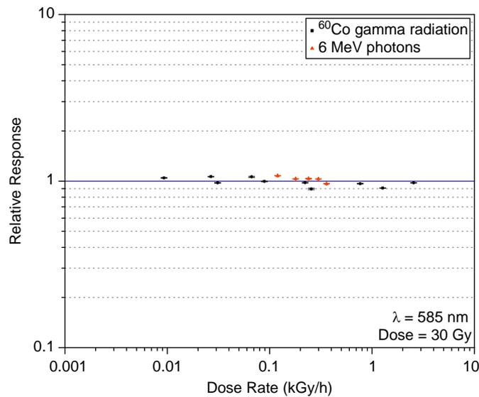
Fig. 2. Spectrophotometric response relative to the mean value of the FXG solutions as a function of dose rate.
