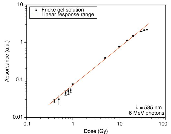
Fig. 6. Spectrophotometric dose response of the Fricke gel solution as a function of absorbed dose.
