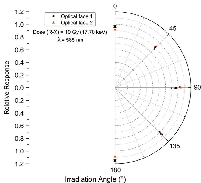
Fig. 3. Spectrophotometric angle dependent response relative to the mean value of the Fricke gel samples of 17.70 keV X-rays.
