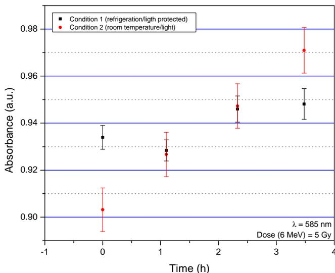
Fig. 5. Spectrophotometric response stability of the irradiated Fricke gel solution in the first 4 h after irradiation.
