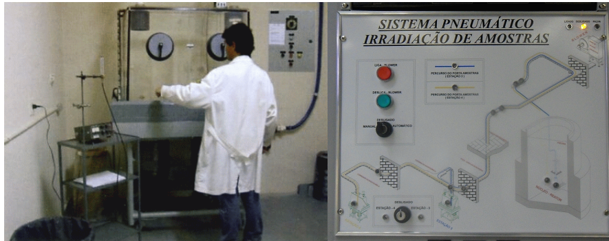
Figure 4. Pneumatic irradiation system, user station (left) and control panel (right).
